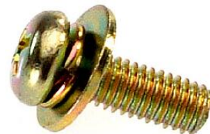
Figure 4. SEMS Screw (Size M3, Spring Washer 5.0Φ, Plain Washer 7.5Φ)
