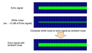
Figure 5. Echo Signal with Ambient Noise
