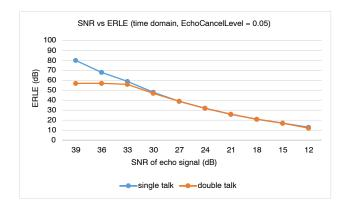
Figure 23. Ambient Noise vs ERLE (Time Domain, Echo Cancel Level = 0.05)
