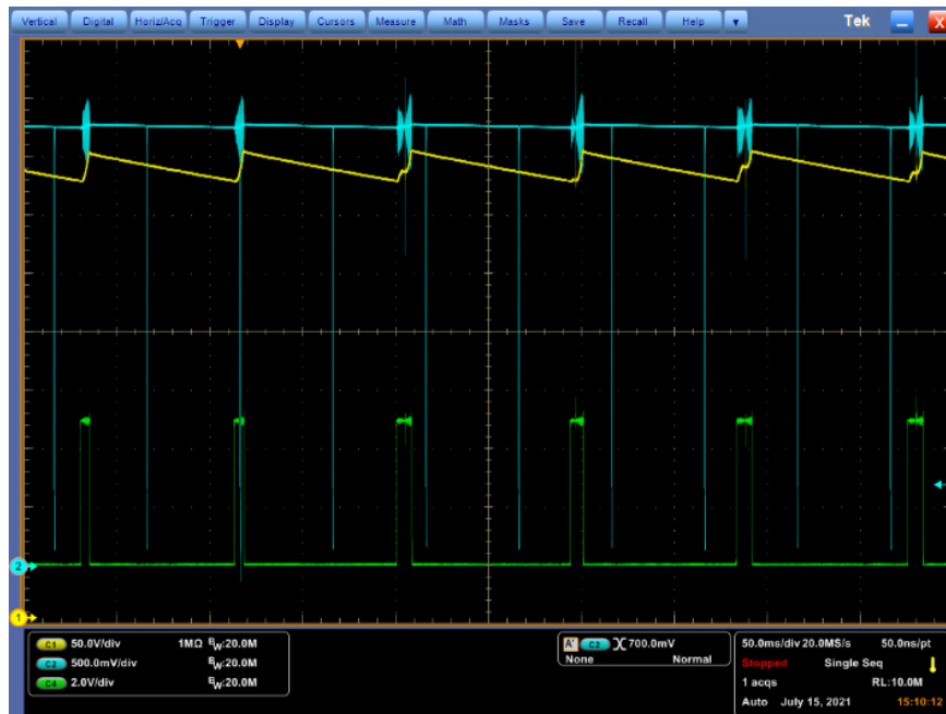
Figure 8. NCP1680 Skip Mode Operation (Ch1 = Bulk Voltage, Ch2 = PFCOK, Ch4 = SKIP)
