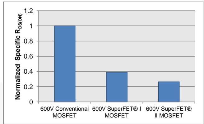
Figure 2. Normalized on-resistance per specific area comparisons
