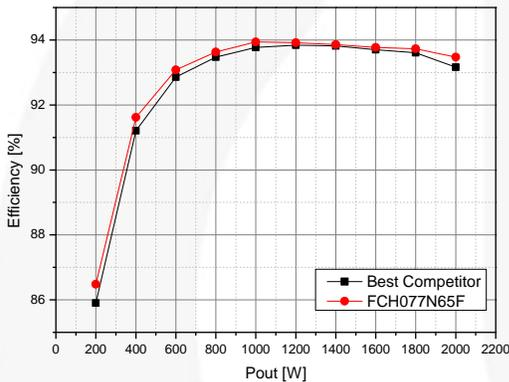
**Figure 15. Efficiency versus output power in 2 kW telecom power supply between SuperFET<sup>®</sup> II FRFET<sup>®</sup> MOSFET, FCH077N65F and 650 V, 80 mΩ competitor's fast recovery MOSFET**
