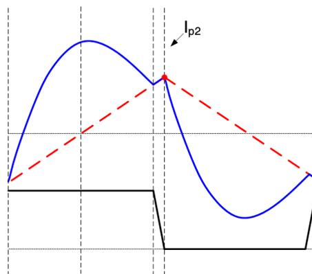
**(b) Waveforms with Small  $L_m$  ( $f_s < f_r$ )**
