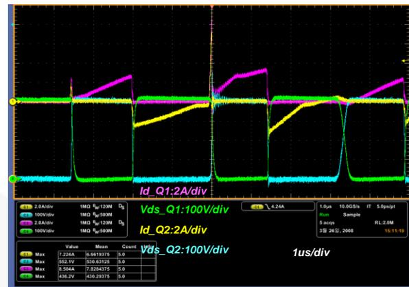
Figure 9. Waveforms of Power MOSFETs at Start-up
