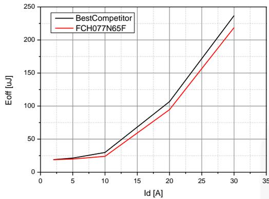
**Figure 14. Turn-off Loss Comparison between SuperFET<sup>®</sup> II FRFET<sup>®</sup> MOSFET, FCH077N65F and 650 V, 80 mΩ competitor's fast recovery MOSFET**
