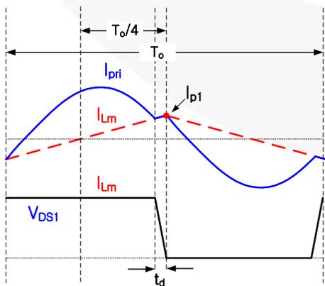
**(a) Waveforms with Large  $L_m$  ( $f_s < f_r$ )**
