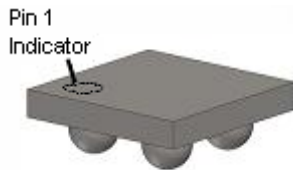
Figure 3. WLCSP Bumps Facing Down (Top View)
