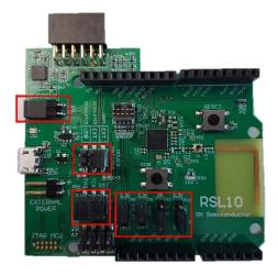
Do not forget to insert a coin cell into the battery holder at the back of the evaluation board. Please note, when the power source of QFN RSL10 evaluation board is a coin cell battery the LED is disabled and the only indication for advertising of beacons is the notification on the smartphone.
