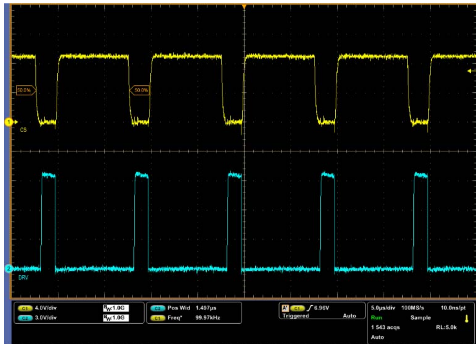
Figure 4: V_{CC} = 12\text{ V} , f = 100\text{ kHz} , DC = 90\% , V_{LOW} = -1\text{ V} , V_{HIGH} = 9\text{ V}
