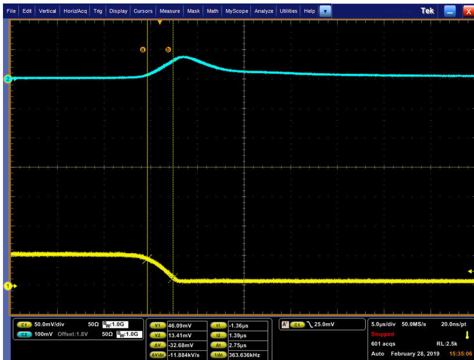
Figure 6: Load step from 125mA to 0A at 10kHz frequency.
