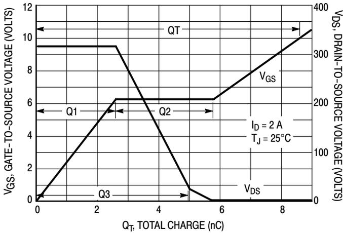
Figure 7. Gate-to-Source and Drain-to-Source Voltage versus Total Charge
