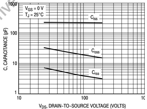
**Figure 1b. High Voltage Capacitance Variation**
