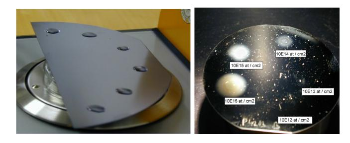
The MCC method starts with intentional contamination of the wafer front
