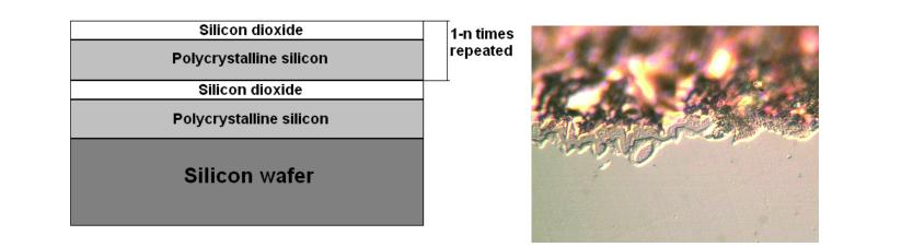
POLY layers enhance the gettering capability of a semiconductor wafer by about two orders of magnitude (measured by MCC) and it is efficient for gettering of heavy metals. However, after each high temperature annealing during the device fabrication process POLY layers losses a great part of its gettering capability.
