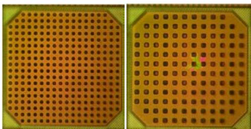
**Figure 7. Designs with arrays of holes in MT(-1) as seen in the cratering test. Both patterns reduced cracks from harsh probing as compared to traditional pads.**
