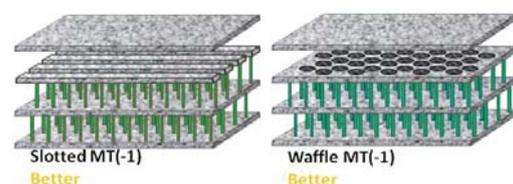
**Figure 5. Illustrations of bond pad structures having: (left) slots in MT(-1), (right) array of holes in MT(-1).**
