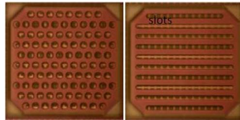
**Figure 9. MT(-1) designs, with different patterns below in MT(-2); (left) MT(-1) array of large holes, (right) MT(-1) slotted metal.**
