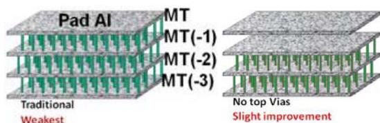
**Figure 3. Illustration of a 4-level metal traditional style bond pads; (left) with top vias, (right) without top vias.**
