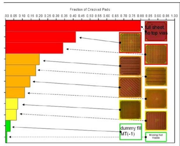
**Figure 13. Chart showing the % of pads cracked for various MT(-1) patterns, worst for full sheet MT(-1) and best for MT(-1) absent from the pad window.**
