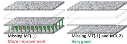
**Figure 4. Illustration of bond pad structures having: (left) MT(-1) absent in the pad window, and (right) both MT(-1) and MT(-2) absent.**
