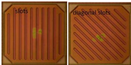
**Figure 6. Examples of slot patterns in MT(-1) as seen in the cratering test. Note the cracks from probing and evidence of etching in the sheet MT(-1). (Left) slots parallel to the probe scrub direction, (right) diagonal slots.**
