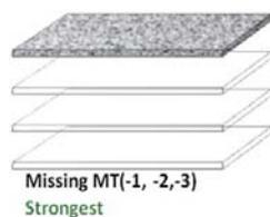
**Figure 12. Illustration of a bond pad structure where all metal sub-layers are absent in the pad window.**
