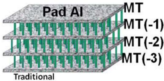
**Figure 1.** Illustration in concept of a traditional bond pad structure, 4 levels of Al-based metallization in this example. W vias electrically connect the full sheets of metal through SiO<sub>2</sub> dielectric that encases everything except the Pad Al surface at the top.
