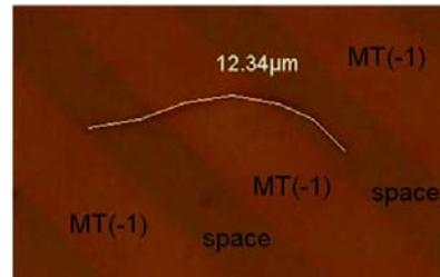
**Figure 16.** Photo of a crack (highlighted in white) above a MT(-1) pattern with diagonal metal lines of 4 $\mu$ m width. Harsh probe scrub direction is down.
