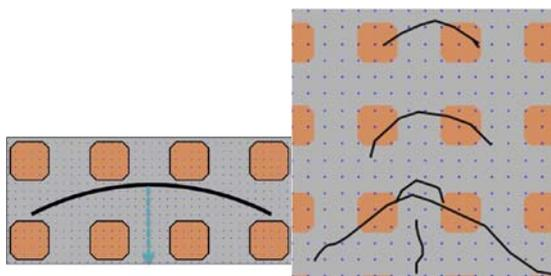
**Figure 18. (left) probe tip heel shape, (right) cracks in a pad initiating over the MT(-1) and changing propagation direction due to interaction with the "holes".**
