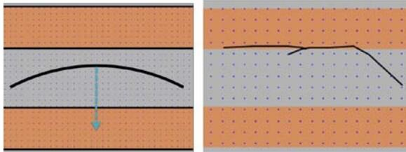
**Figure 14.** Top view illustrations of: (left) a typical crack shape expected from the probe tip over wide MT(-1) [gray color], (right) image of an actual crack initiating at the point where the MT(-1) line begins. Brown color represents the SiO<sub>2</sub>. The cantilever probe scrub direction is downward. (Small dots on the illustrations are not vias, they are just grid points).
