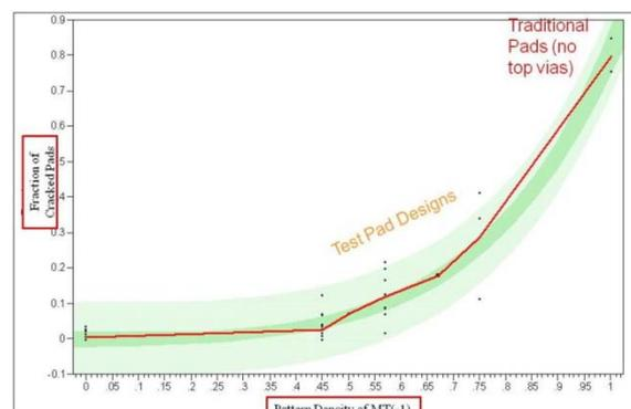
**Figure 2.** Fraction of pads that cracked vs MT(-1) pattern density in the pad window
