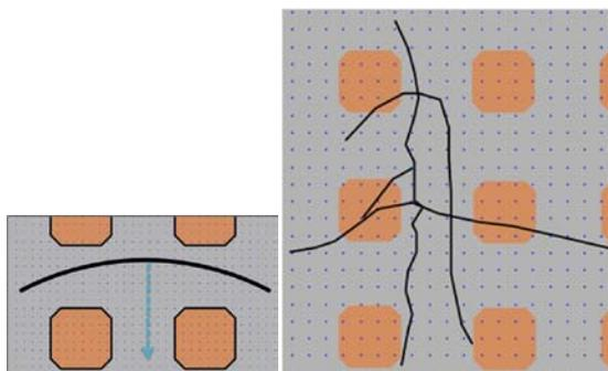
**Figure 17. (left) probe heel tip shape drawn over a MT(-1) pattern with an array of holes, (right) actual crack shapes from one harshly probed pad, initiating over the MT(-1) and propagating in various directions due to interaction with the “holes”.**
