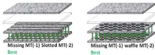
**Figure 11. Illustration of bond pad structures having MT(-1) absent, and: (left) slotted MT(-2) and MT(-3), (right) array of holes in MT(-2) and MT(-3).**
