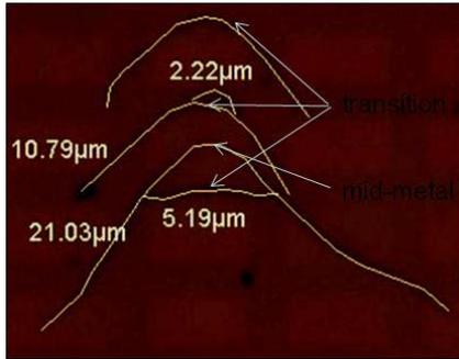
**Figure 21. Cracks above MT(-1) dummy fill pattern. Cracks initiate only at the transition from space to metal, or in the center of the metal.**
