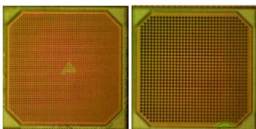
**Figure 8. Designs with arrays of smaller holes in MT(-1) as seen in the cratering test. Both test patterns have the same metal width between holes, but the pattern on the right prevented cracks best in harsh probing, having wider holes and less overall metal density.**
