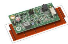
Left: Figure 1. The RSL10 Solar Cell Multi-Sensor Platform with attached solar panel and ready to transmit sensor data over Bluetooth Low Energy (BLE)
