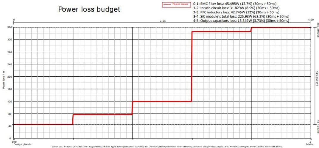
Fig. 12. An example of a power loss budget. Main conditions for this simulation are V_{IN} = 230\text{ V} , P_{OUT} = 26.5\text{ kW} , V_{OUT} = 800\text{ V} and the inductor and capacitor set = 245\text{ }\mu\text{H} and 4 \times 470\text{ }\mu\text{F} . Simulation time is 50 ms. Time window considered for the energy loss (power loss) computation is from 30 ms to 50 ms (as indicated by "30ms % 50 ms" in the key), in order for the system to be running in steady state.
