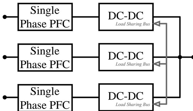
Fig. 17. Three-phase PFC using three single-phase PFC stages.
