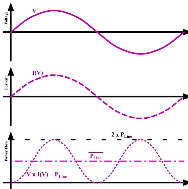
Fig. 2. Power flow from a single-phase grid.
