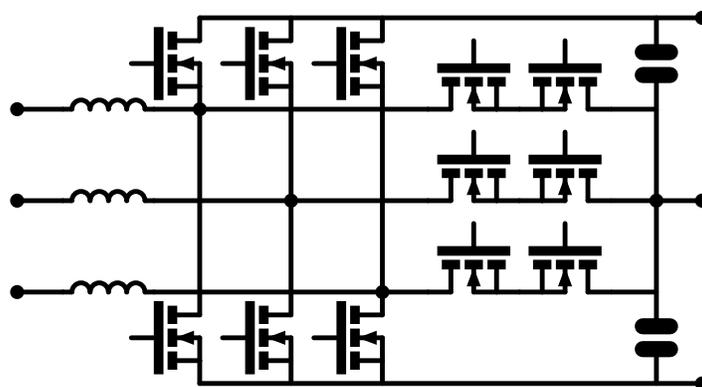
Fig. 11. Bidirectional T-NPC boost PFC schematic.
