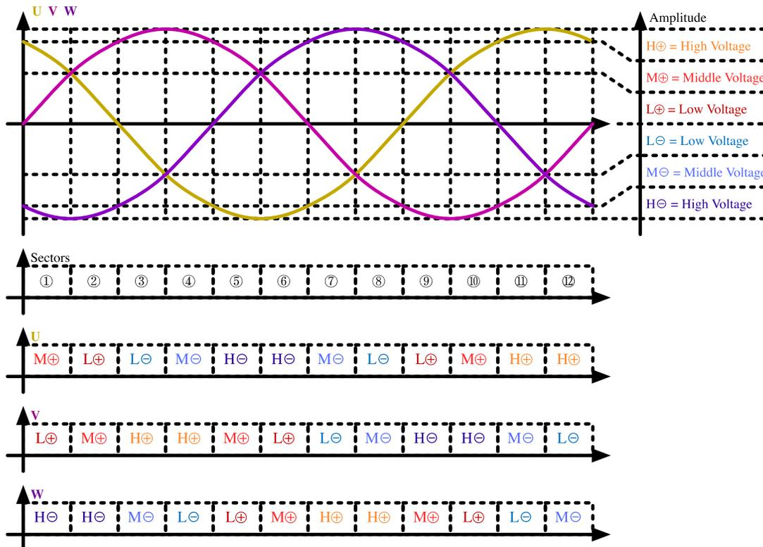
Fig. 6. Three-phase voltages and sectors.
