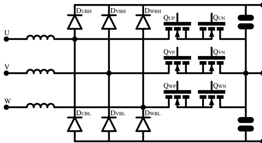
Fig. 9. T-NPC boost PFC schematic.
