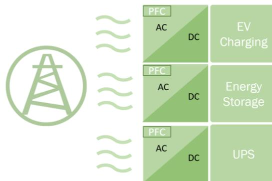
Fig. 1. EV charging is accelerating the need for three-phase-based PFC for ac-dc conversion. Other applications that are driving its implementation are energy storage systems (ESSs) and uninterruptible power supplies (UPSs) for industrial sites and data centers.
