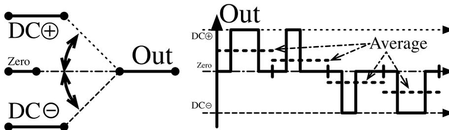
Fig. 5. Bipolar or three-level switching principle.
