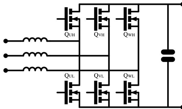
Fig. 15. Six-switch bidirectional two-level boost PFC schematic.
