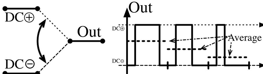
Fig. 4. Unipolar or two-level switching principle.
