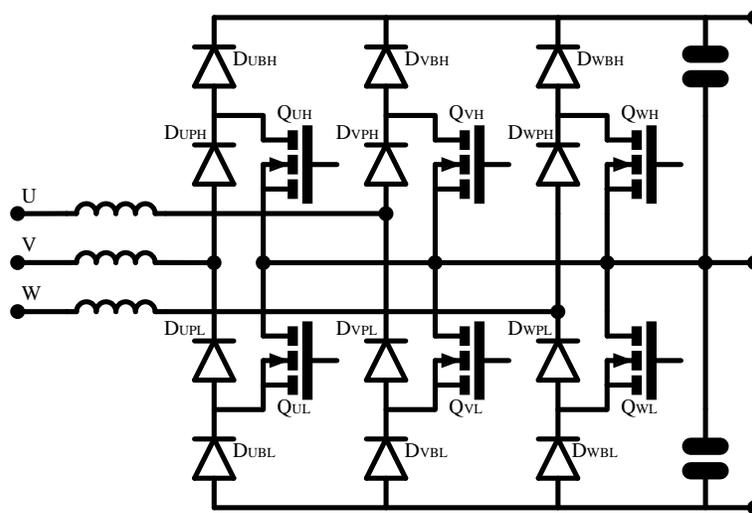
Fig. 12. NPC boost PFC schematic.
