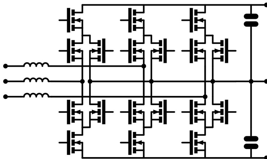
Fig. 14. Bidirectional NPC boost PFC schematic, also called A-NPC boost PFC.
