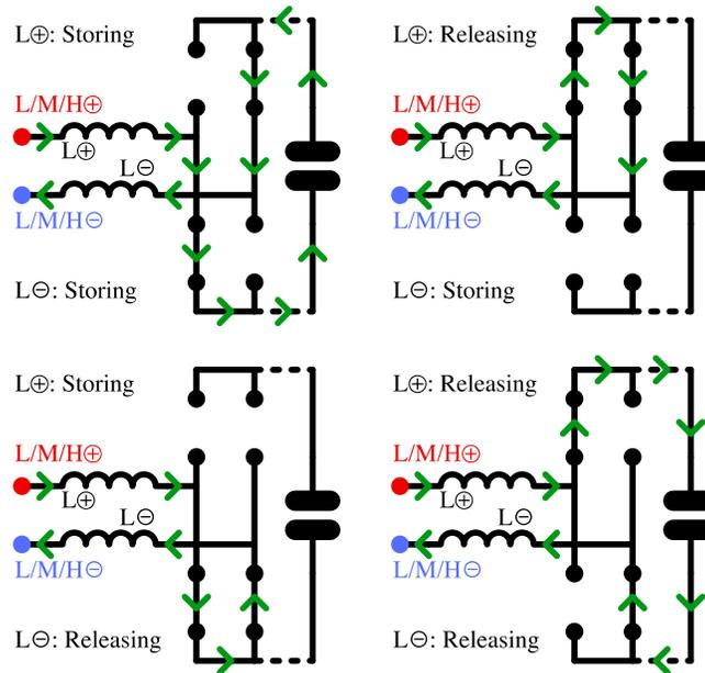
Fig. 16. Six-switch boost PFC current paths for energy storing and energy releasing (boosting) modes and phase voltage.
