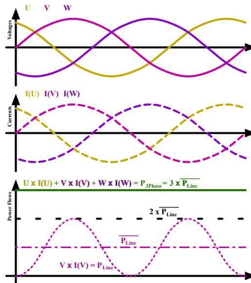
Fig. 3. Power flow from a three-phase grid.
