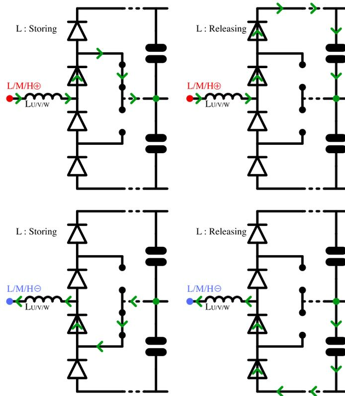
Fig. 13. NPC boost PFC current paths (for energy storing and energy releasing modes) and phase voltage.
