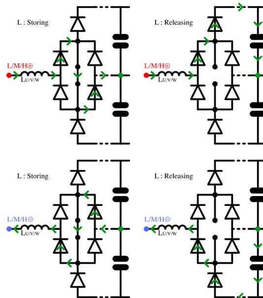
Fig. 8. Vienna boost PFC current paths (for energy storing and energy releasing modes) and phase voltage.
