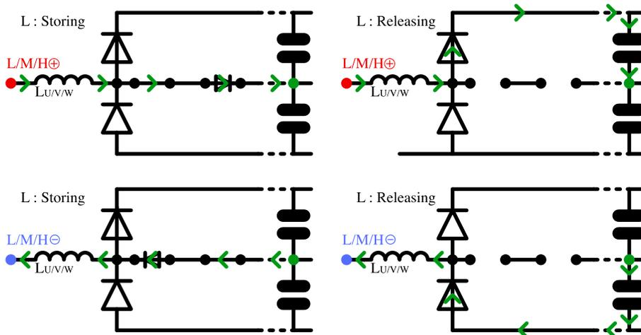
Fig. 10. T-NPC boost PFC current paths (for the storing and releasing energy modes) and phase voltage.
