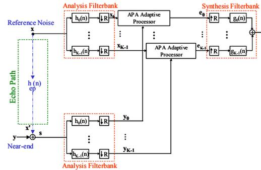
Figure 1: Block diagram of the OS-SAF system.
