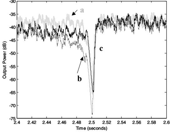
Figure 3: Output power in time for: (a) grey-thick line,  $\delta = 5 \times 10^7$ ,  $\mu = 0.7$ ,  $L = 24$ , (b) dashed line,  $\delta = 5 \times 10^7$ ,  $\mu = 0.7$ ,  $L = 96$ , (c) black-thin line,  $\delta = 2.5 \times 10^8$ ,  $\mu = 1.575$ ,  $L = 96$ .
