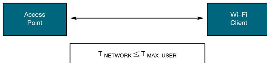
In these legacy Wi-Fi networks, consider two scenarios for doing speed test. In the first scenario, multiple devices are connected and are all simultaneously trying to do the speed test and in the second scenario, only a single device, the one with maximum throughput is connected and performing the speed test. The total aggregated throughput in first scenario will be definitely lower than the second one.
