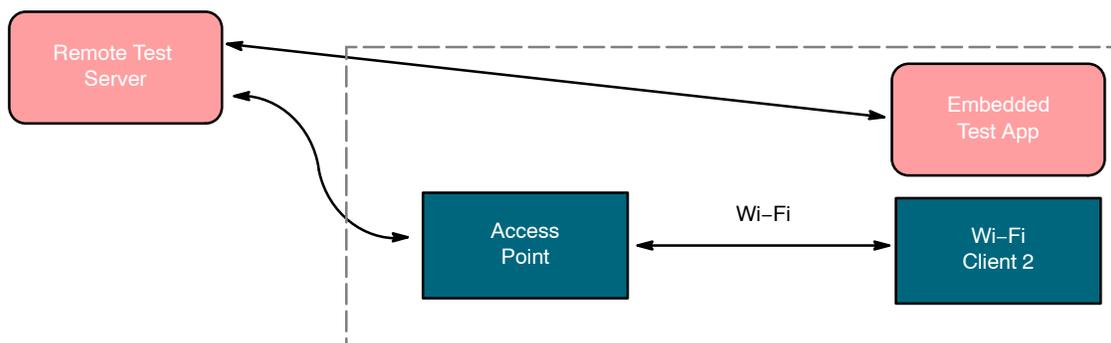
To properly isolate the Wi-Fi performance from the broadband speed, it is necessary to use a local test server attached to the access point, as illustrated below. Using traffic generation tools such as iPerf or Chariot to allow for accurate testing of Wi-Fi only traffic.
