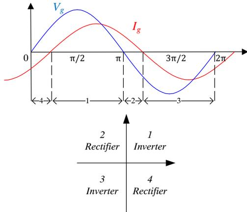
**Figure 28. Half-bridge Four-quadrants Operations**
