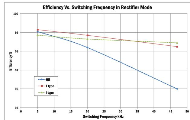
**Figure 35. Efficiency versus Switching Frequency in Rectifier Mode. Comparison between an HB, I-Type and T-Type [14]**
