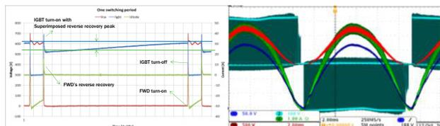
**Figure 30. Switching Waveforms in Motor Drive Applications**
