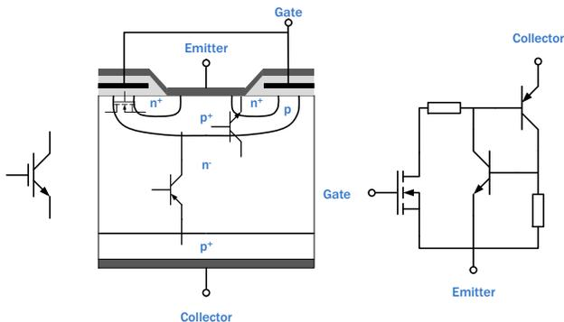
Figure 4. IGBT with Parasitic Structure
