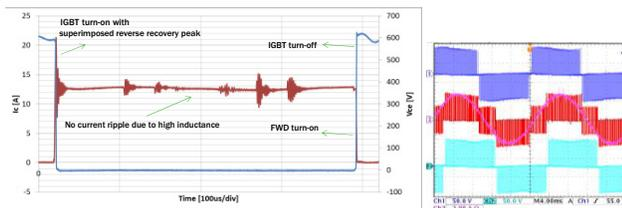
**Figure 29. Switching Waveforms in Motor Drive Applications**
