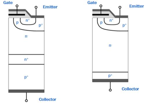
Figure 5. Left) Punch-through (PT) IGBT; Right) Non-punch-through (NPT) IGBT
