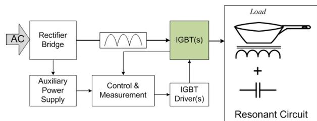
**Figure 19. System Block Diagram of Welding Machines**
