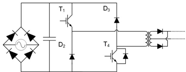
**Figure 15. Double Switches Forward Topology**
