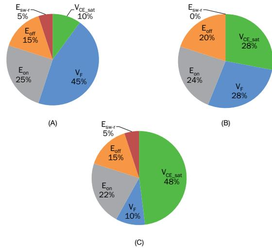
**Figure 36. Losses Distribution of a Given IGBT Operating in the Vienna Topology, Half-bridge and Full-bridge**
