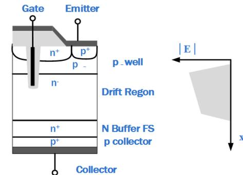
Figure 6. Field Trench Stop IGBT Structure
