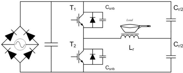
**Figure 20. Resonant Half-bridge Topology for Induction Cooking Applications**
