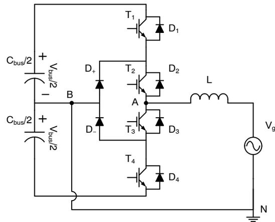
**Figure 31. I-Type Converter**
