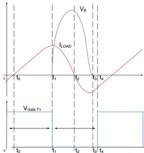
**Figure 23. QR Single – End Inverter and its Associated Waveforms**
