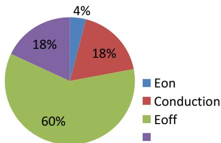
**Figure 18. IGBT Losses Distribution in a Full-bridge Welding Machine 5 kW. Nominal ac 230 V Input. Output Current Full Load (250 A)**
