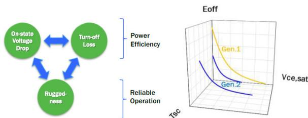
Figure 8. Left) The IGBT Triangle; Right) Trade Off Relationship
