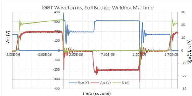
**Figure 12. Waveform of a Full-bridge Welding Machine**
