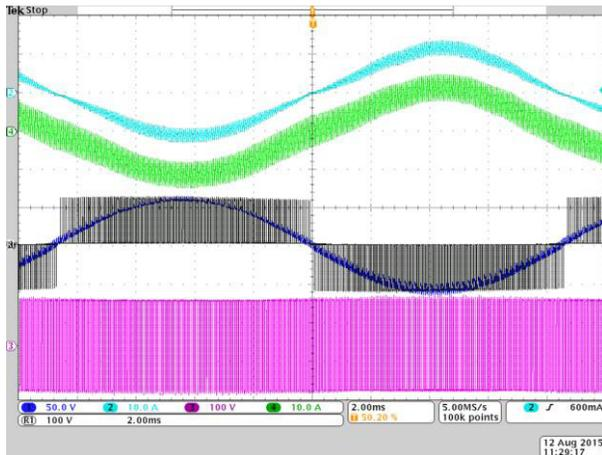
**Figure 33. Comparison between a Classical Half-bridge and a Three-level Converter in Terms of Voltage and Current Output**
