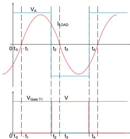
**Figure 21. Resonant Half-bridge Inverter and its Waveforms**
