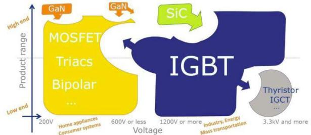
Figure 1. Power Switch Environment [1]
