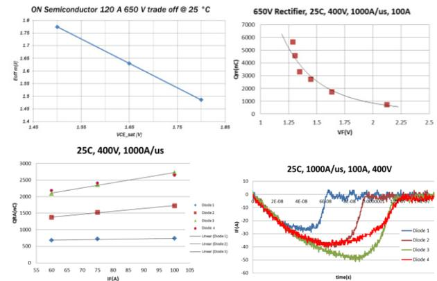
Figure 9. Examples of IGBT and Antiparallel Diode Possible Trade Off
