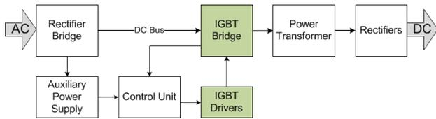
**Figure 10. System Block Diagram of Welding Machines**
