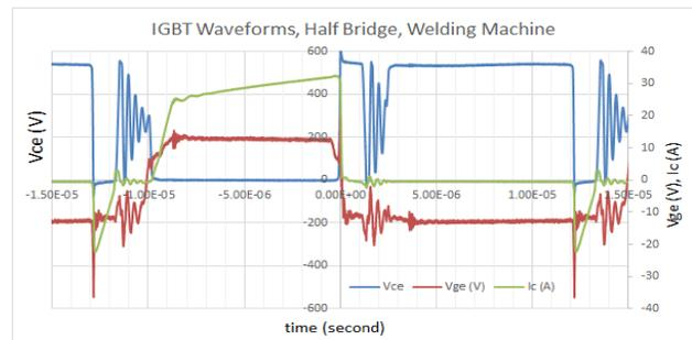
**Figure 14. Waveform of a Half-bridge Welding Machine**
