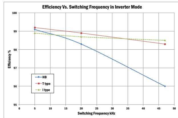
**Figure 34. Efficiency versus Switching Frequency in Inverter Mode. Comparison between an HB, I-Type and T-Type [14]**
