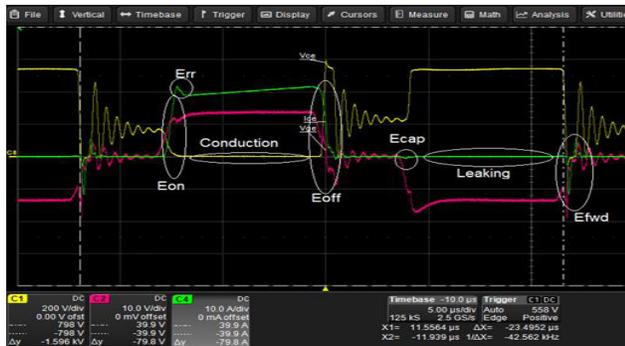
**Figure 17. Switching Waveforms for a Full-bridge Welding Machine**
