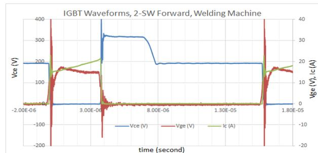
**Figure 16. Waveform of a Two-switch Forward Welding Machine**
