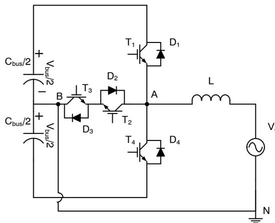
**Figure 32. T-Type Converter**
