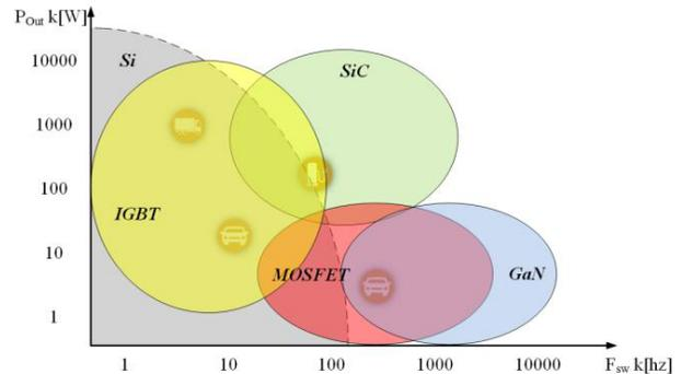
Figure 2. Range of Operation of Silicon and Wide Band Gap Devices
