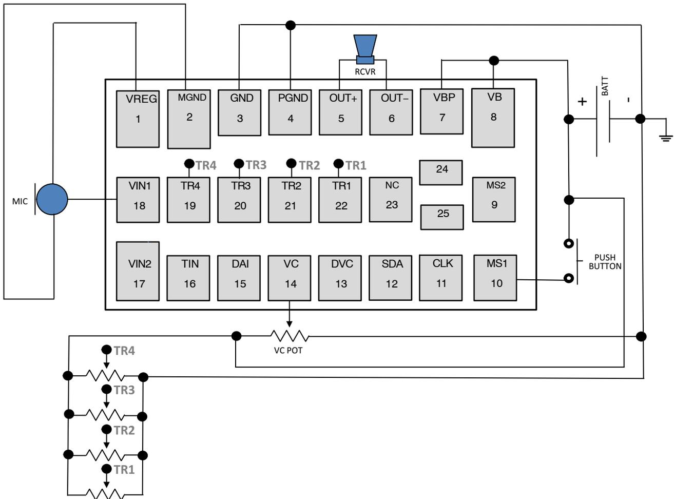
**Figure 4. BTE Schematic Diagram**
