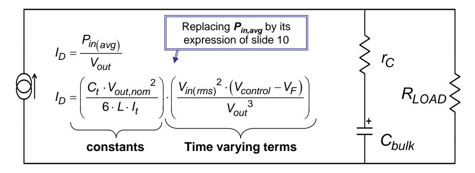
• 3 sources of perturbations:  $V_{CONTROL}$ ,  $V_{out}$  and  $V_{in(rms)}$ .
