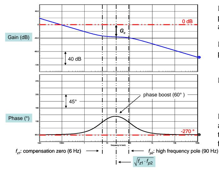
$\Box$   $f_{p2}$  and  $f_{z1}$  set the phase boost magnitude and location (frequency)
