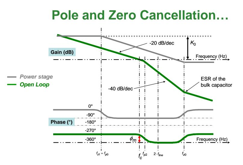
□ The higher  $f_{p2}$ , the larger the phase margin □ The lower  $f_{p2}$ , the better the rejection of the low frequency ripple □  $\phi_m = 45^\circ$  if  $f_{p2} = f_c$ .
