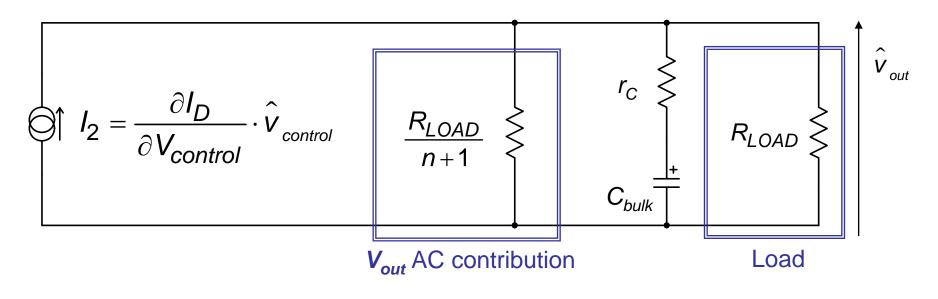
• Noting that:  $\frac{R_{LOAD}}{n+1} \square R_{LOAD} = \frac{R_{LOAD}}{n+2}$
