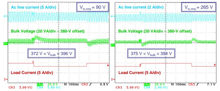
The high-line, larger bandwidth reduces the V<sub>bulk</sub> deviations and speedsup the output voltage recovery
