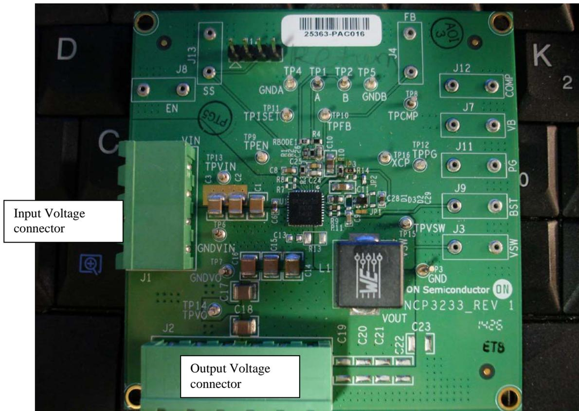
For operation at input voltages greater than 5 V, reverse the prior settings, i.e., open J2 and J3 and short J1, and install the zero- $\Omega$  resistor into R14. The EVB should now be configured to operate from 5 V to the maximum input voltage for the EVB (~21 V).
