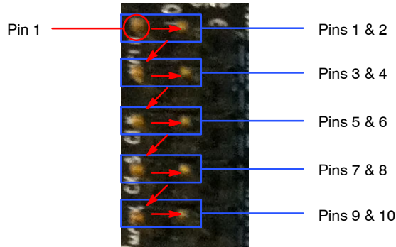
Figure 6. Pin Locations and Assignments of Grouped Jumpers. Pin 1 is Located at the Top-Left Corner and Increases in a Zigzag Fashion Shown in the Picture
