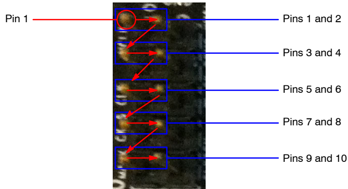
Figure 6. Pin Locations and Assignments of Grouped Jumpers. Pin 1 is Located at the Top-Left Corner and Increases in a Zigzag Fashion Shown in the Picture
