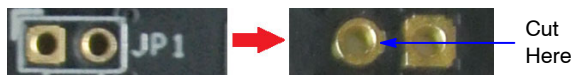
Figure 7. Top and Bottom View of Shorted Jumper. The Bottom View Shows the Trace Location to Cut for Current Measurement
