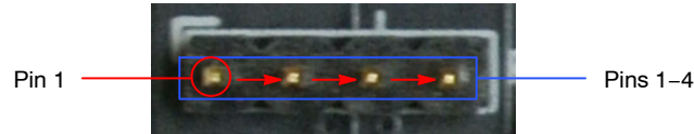
Figure 5. Pin Locations for a Single Jumper. Pin 1 is Located at the Leftmost Side and Increases as it Moves to the Right
