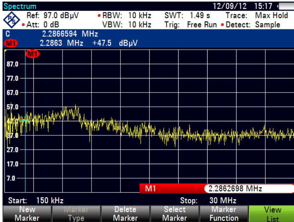
Figure 23. Conducted EMI Pre-compliance 150 kHz–30 MHz
