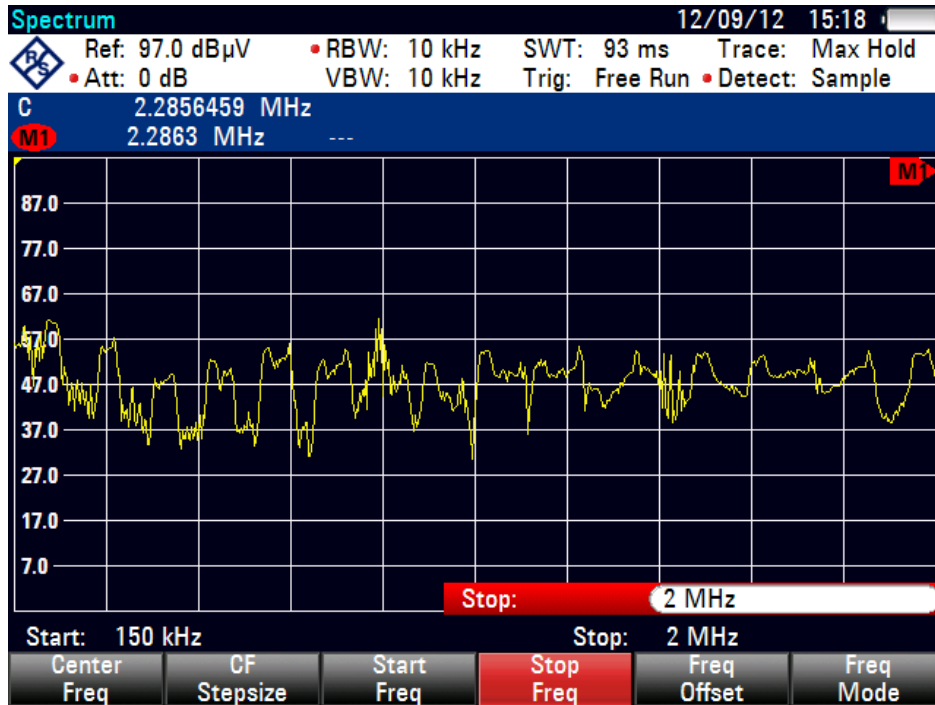
Figure 22. Conducted EMI Pre-compliance 150 kHz–2 MHz
