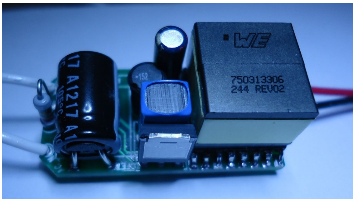
Figure 1. NCL30081LEDG Evaluation Board
