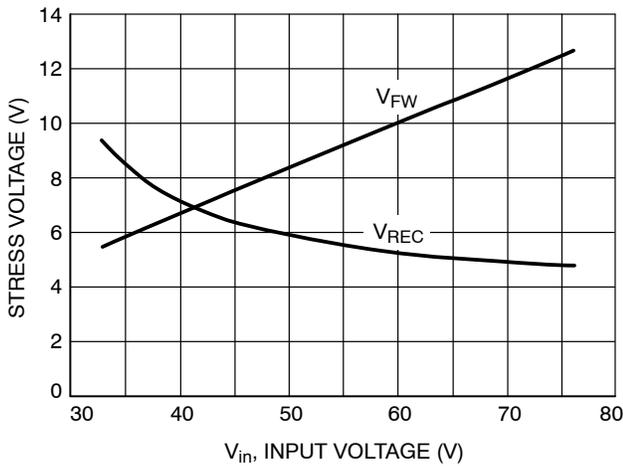
**Figure 12. Synchronous Rectifier Gate Voltage**
