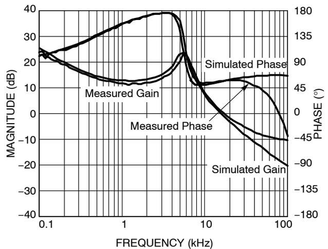
**Figure 30. Measured and Calculated Open Loop Frequency Responses**
