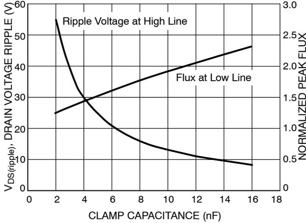
**Figure 6.  $V_{DS(ripple)}$  and Normalized Peak Flux vs.  $C_{clamp}$**
