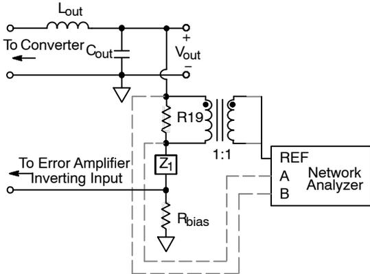
**Figure 29. Open Loop Frequency Response Measurement Setup**
