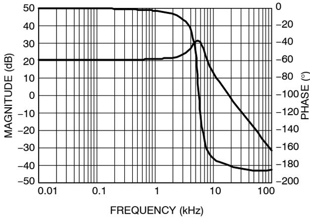
Figure 15. Simulated Open Loop Frequency Response
