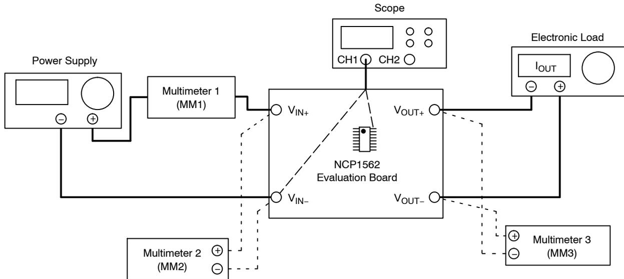
**Figure 38. Test Setup**
