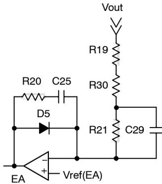
Figure 16. Type II Error Amplifier
