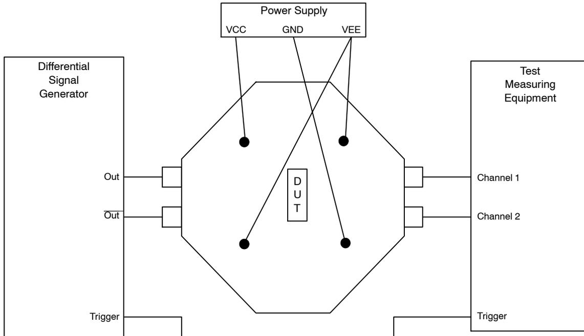
Figure 5. Simplified Equipment Lab Setup Block Diagram
