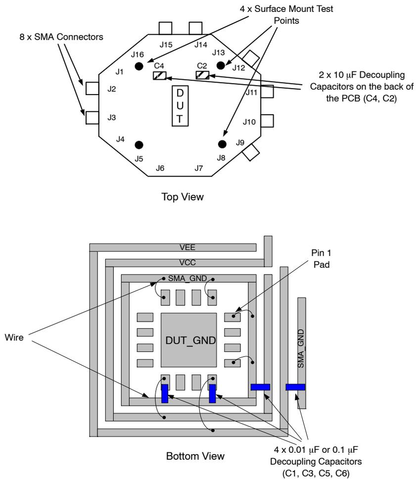
**Figure 3. Components Placement**
