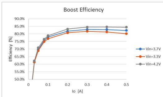
Figure 1: LC709301F boost efficiency based on battery capacity
