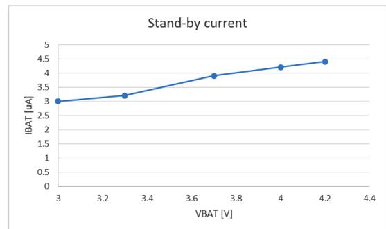
Figure 2: LC709301F standby current including Lib-protection IC
