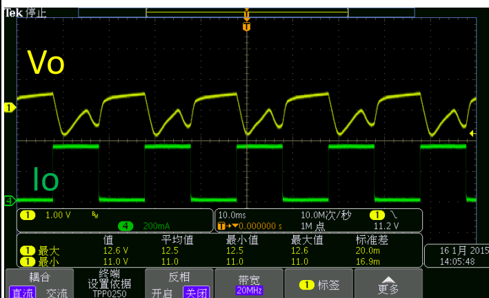
Test Condition: 0-350mA, 100mA/us 20ms cycle, 115Vac
