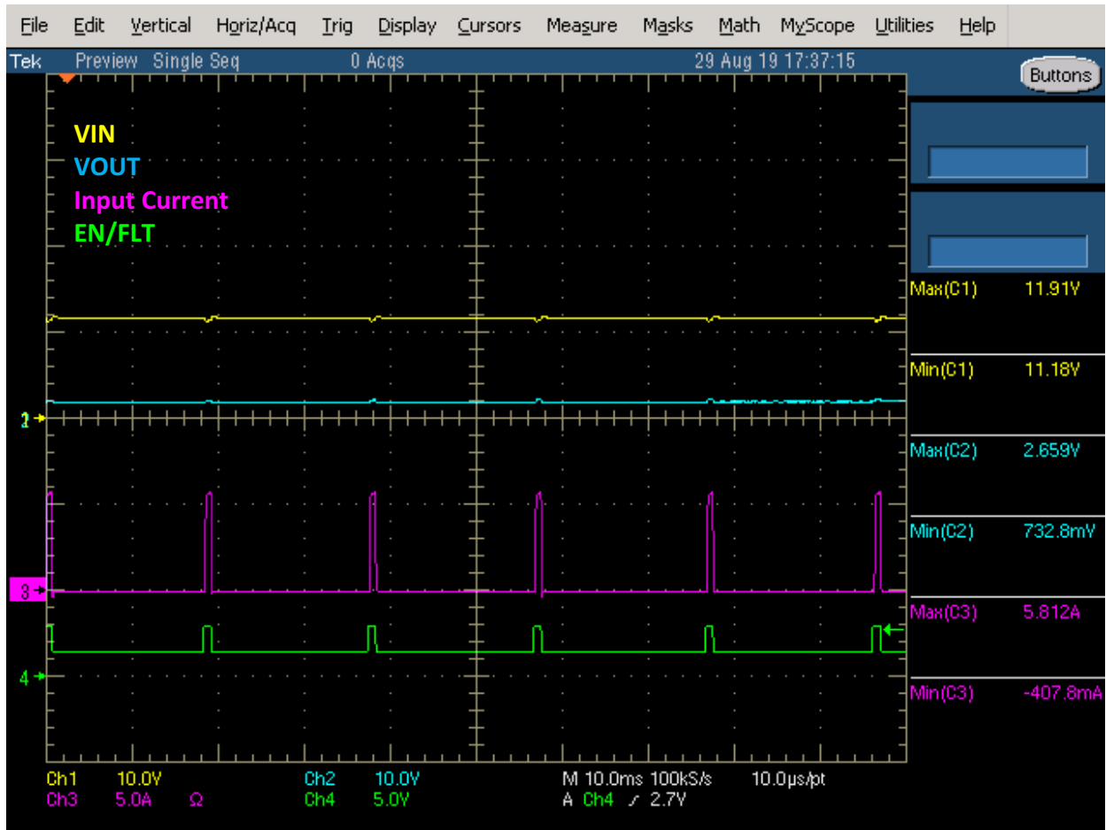
Figure 4. Restart Cycles and Enable/Fault Pin Levels of NIS5020 during Output Capacitance Charging
