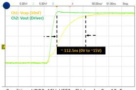
Condition: VDD2=15V, VEE2=-8V, Load =  $C_L$  = 10nF, R<sub>EX</sub> = 2 $\Omega$ , C<sub>EX</sub> = 2.2nF
