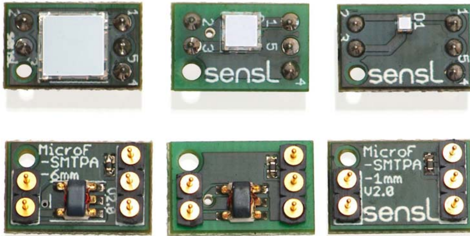
Figure 12. (Top) top view and (bottom) bottom view of the ON Semiconductor SMTPA boards, from left to right 6mm, 3mm and 1mm. The M-, B-, C- and RA-Series versions are all (visually) the same
