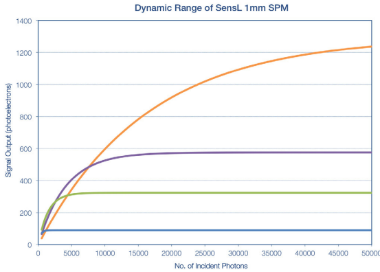
Figure 1. Calculated Values for the Signal Output for Varying Numbers of Incident Photons, for Differing Microcell Sizes (20 μm, 35 μm, 50 μm and 100 μm) on a 1 mm Sensor
