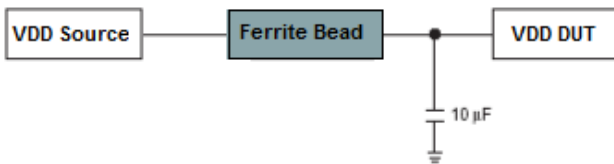
Figure 9. Power Supply Noise Filtering Example
