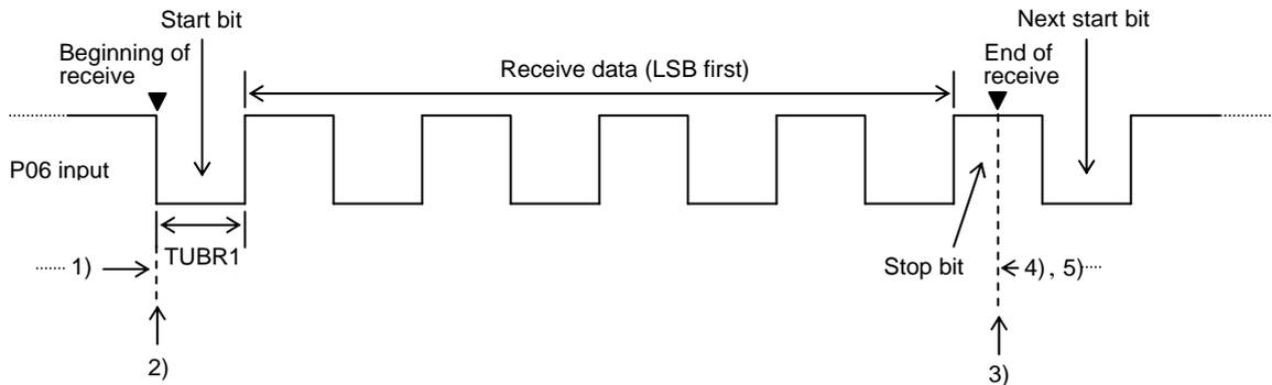
**Figure 3.8.3 Example of Continuous 8-bit Data Receive Mode Processing**
