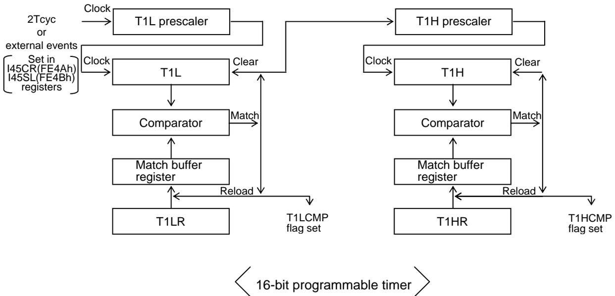
Figure 3.4.2 Mode 2 (T1LONG = 1, T1PWM = 0) Block Diagram
