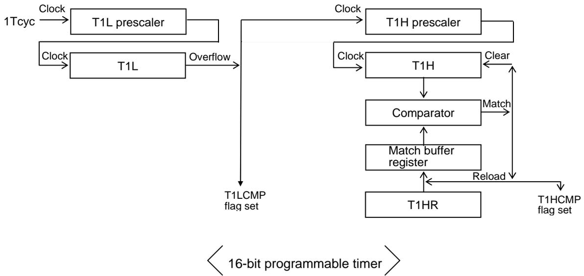
Figure 3.4.3 Mode 3 (T1LONG = 1, T1PWM = 1) Block Diagram
