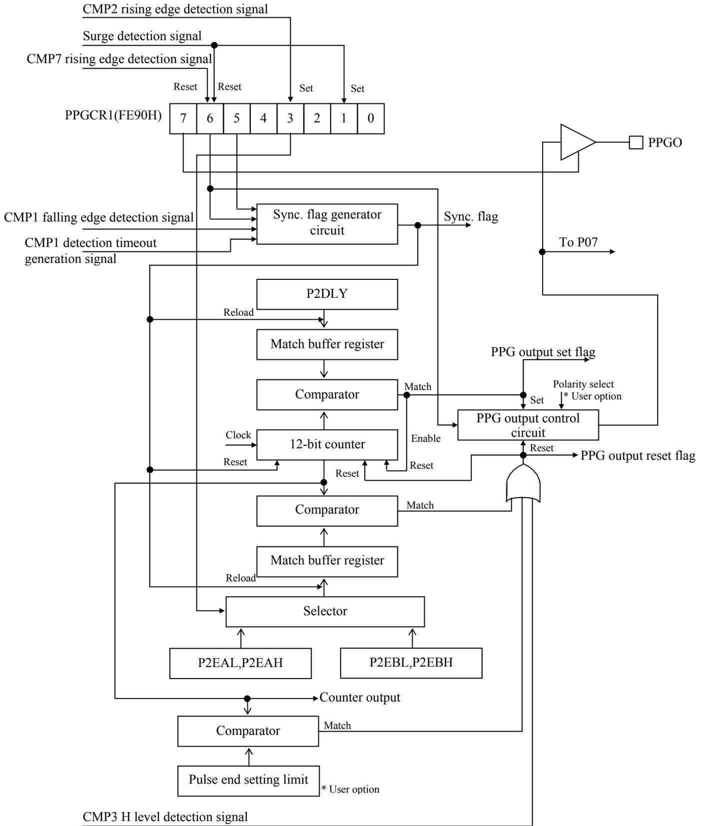
Figure 3.10.3 PPG Block Diagram 1
