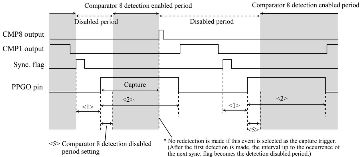
**Figure 3.10.10 PPG Output Timing 5**
