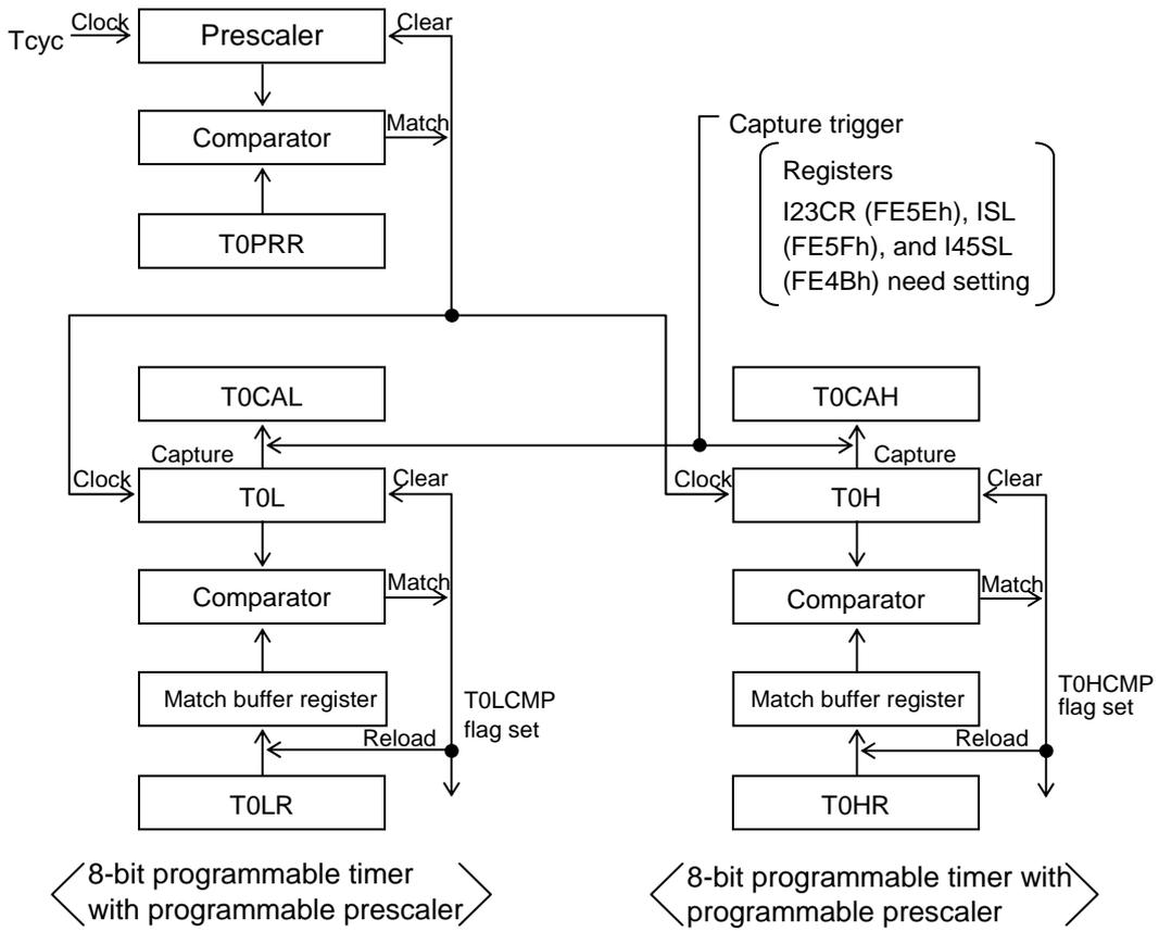
Figure 3.3.1 Mode 0 Block Diagram (T0LONG = 0 , T0LEXT = 0)
