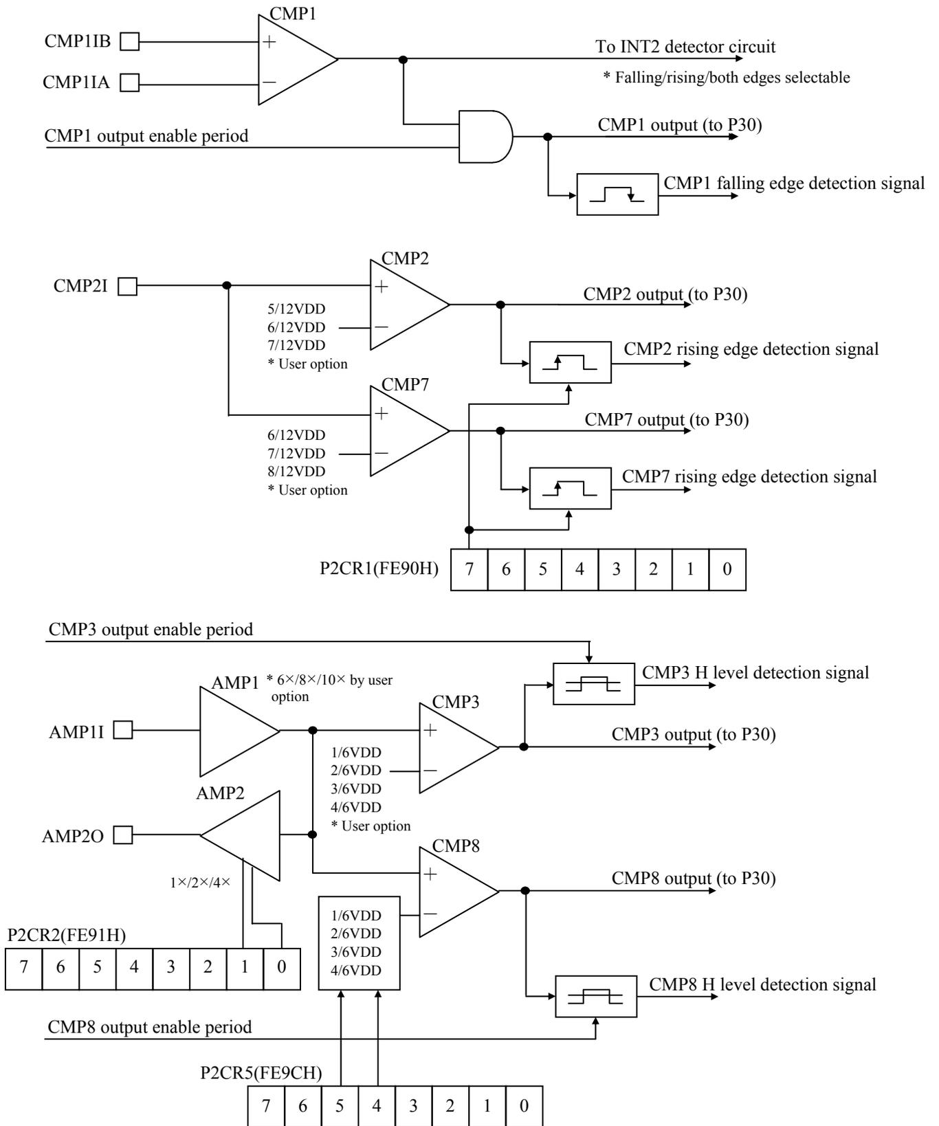
Figure 3.10.1 Amplifier/Comparator Block Diagram
