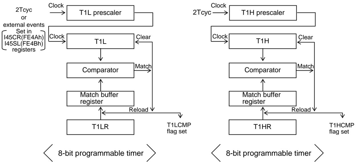
Figure 3.4.1 Mode 0 (T1LONG = 0, T1PWM = 0) Block Diagram
