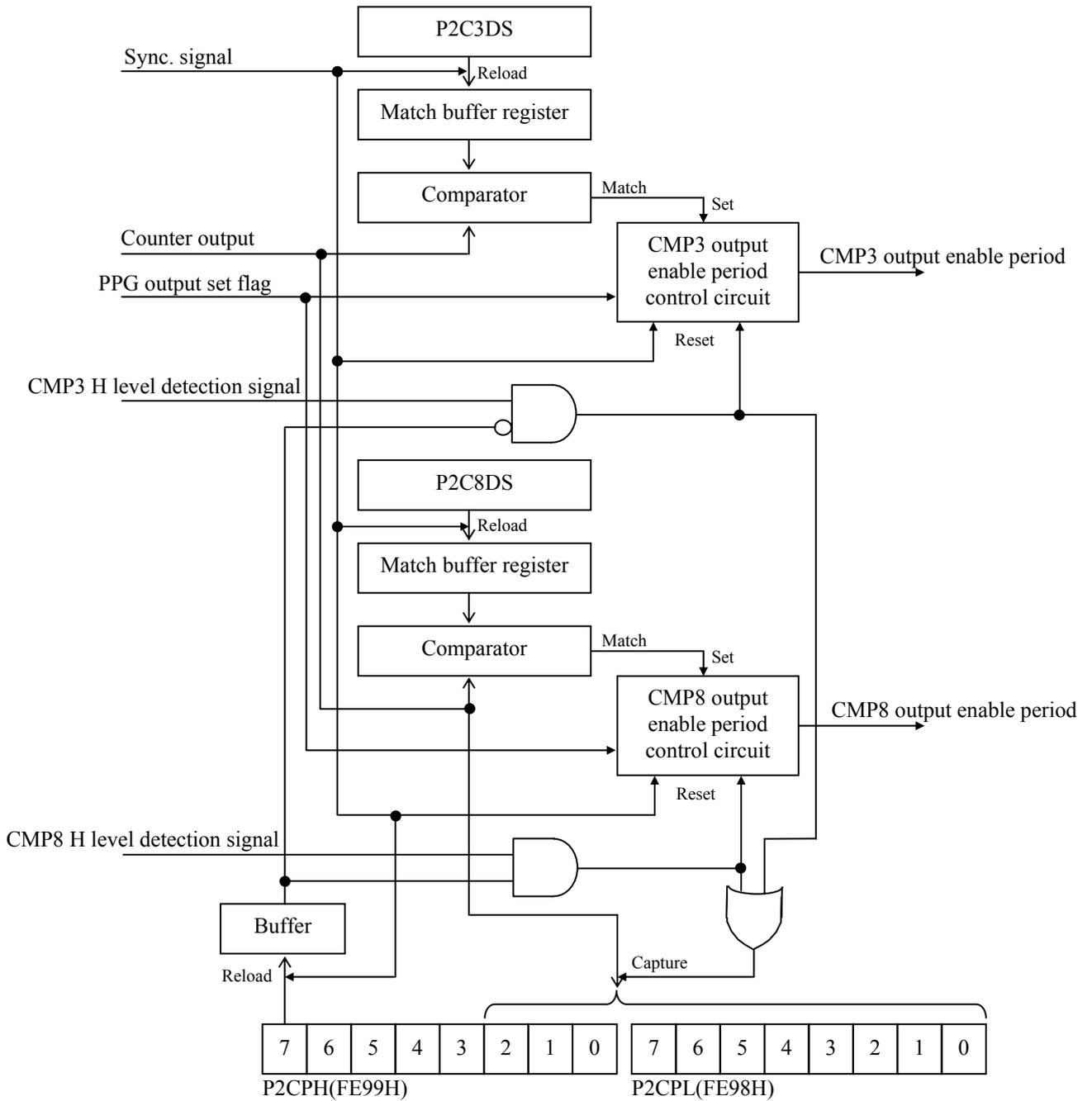
Figure 3.10.5 PPG Block Diagram 3
