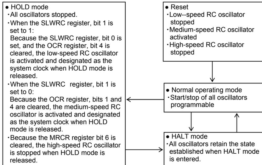
5) It is necessary to manipulate the following special function registers to control the system clock.
