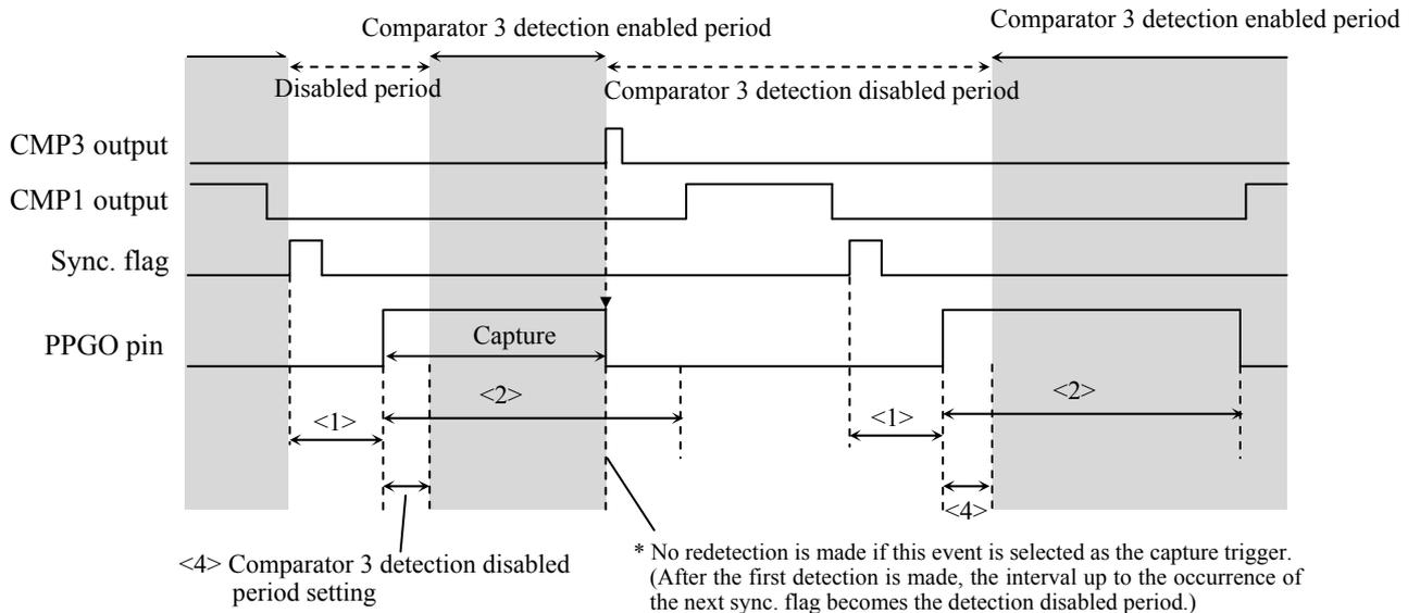
**Figure 3.10.9 PPG Output Timing 4**
