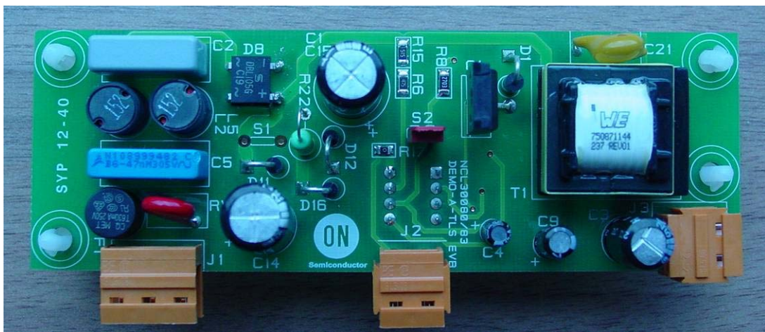
Figure 3. Photograph of the Top Side of the Valley Fill EVB
