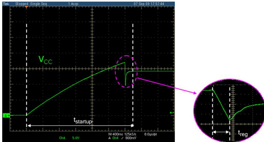
Figure 12.  $V_{CC}$  Waveform during Startup
