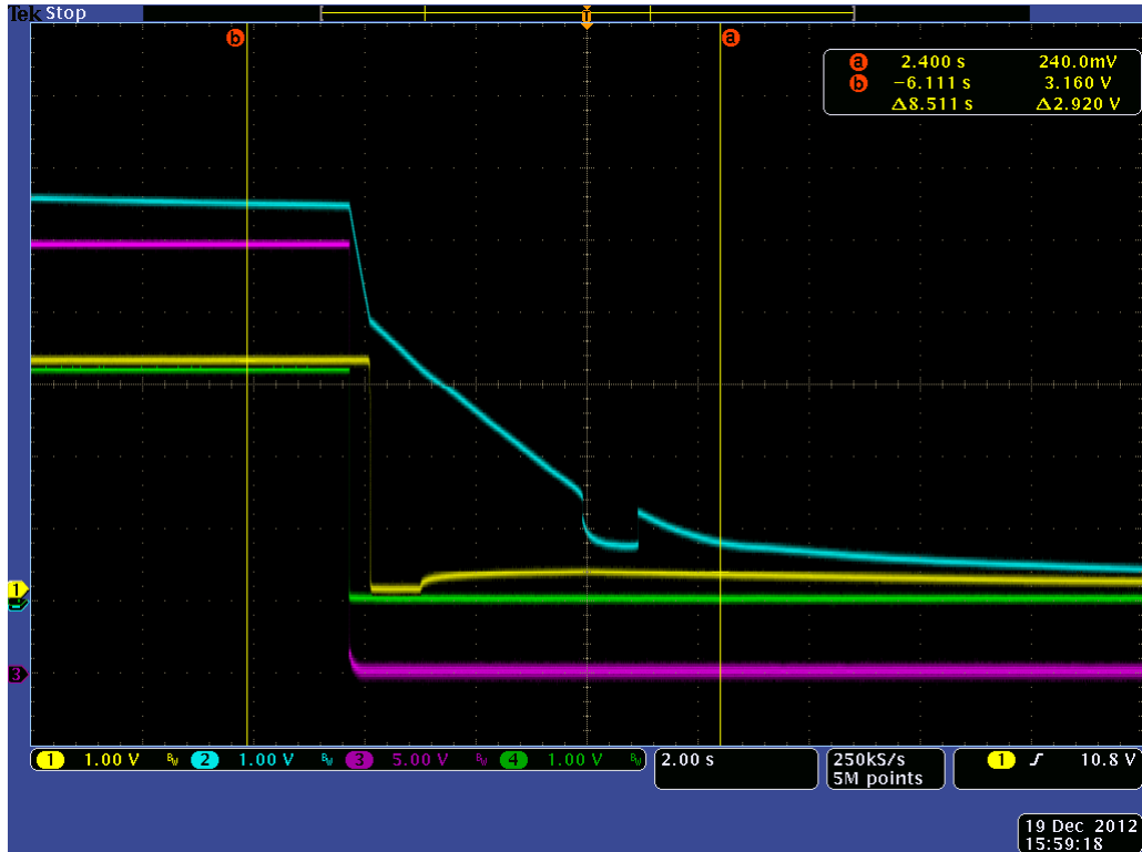
Figure 9. TSS721A Shutdown ( C_{STC} = 220 \mu\text{F} , 1 Unit Load, external load of 8 \text{ k}\Omega disconnected on shutdown) (purple = BUSL1, blue = STC, yellow = VDD, green = PFb)
