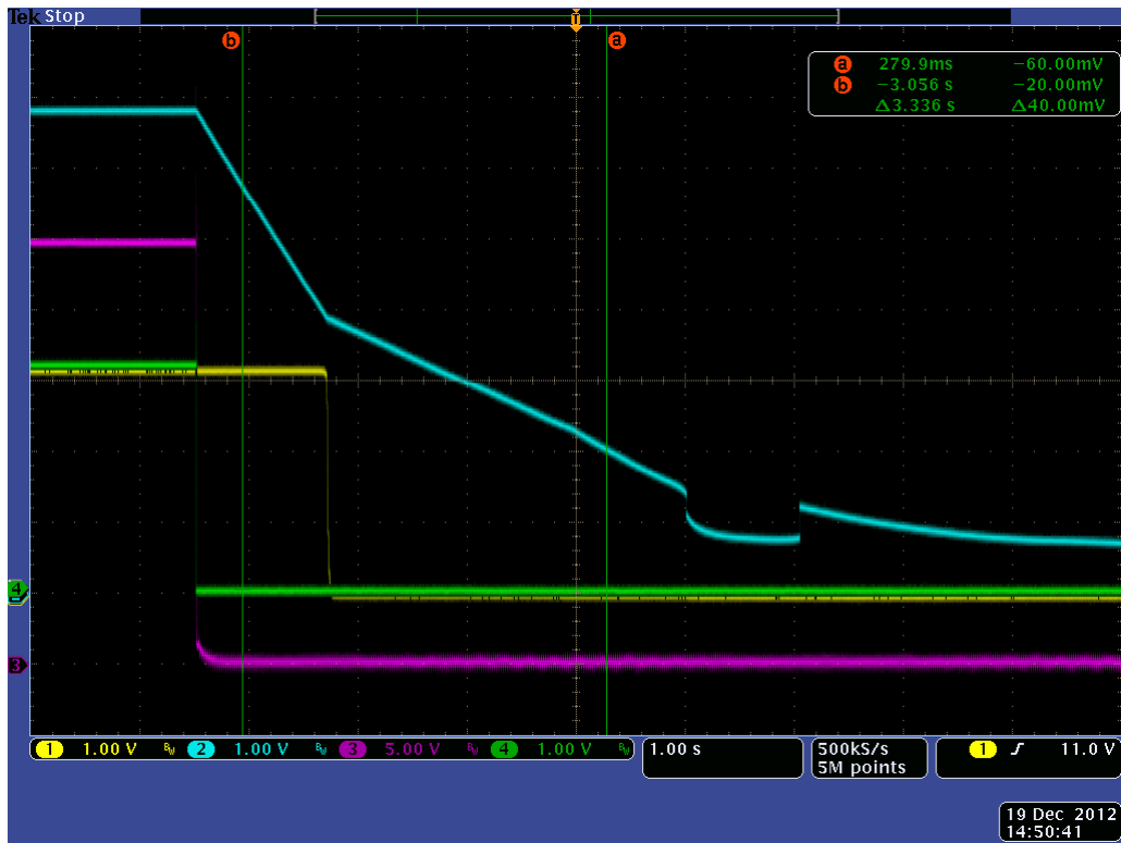
Figure 8. TSS721A Shutdown ( C_{STC} = 220 \mu\text{F} , 1 Unit Load, external load of 8 \text{ k}\Omega ) (purple = BUSL1, blue = STC, yellow = VDD, green = PFb)
