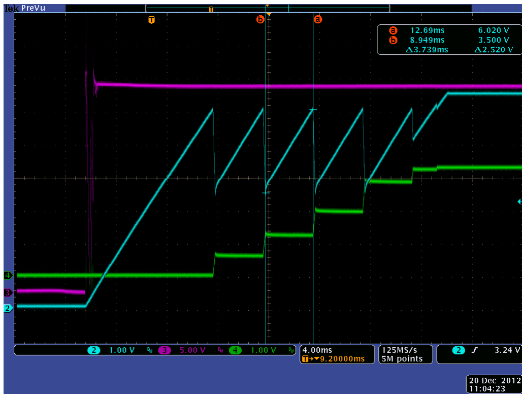
Figure 10. Charge Transfer Instability (NCN5150, C_{STC} = 2 \mu F , C_{VDD} = 1 \mu F , 1 Unit Load, no external load) (purple = BUSL1, blue = STC, green = VDD)
