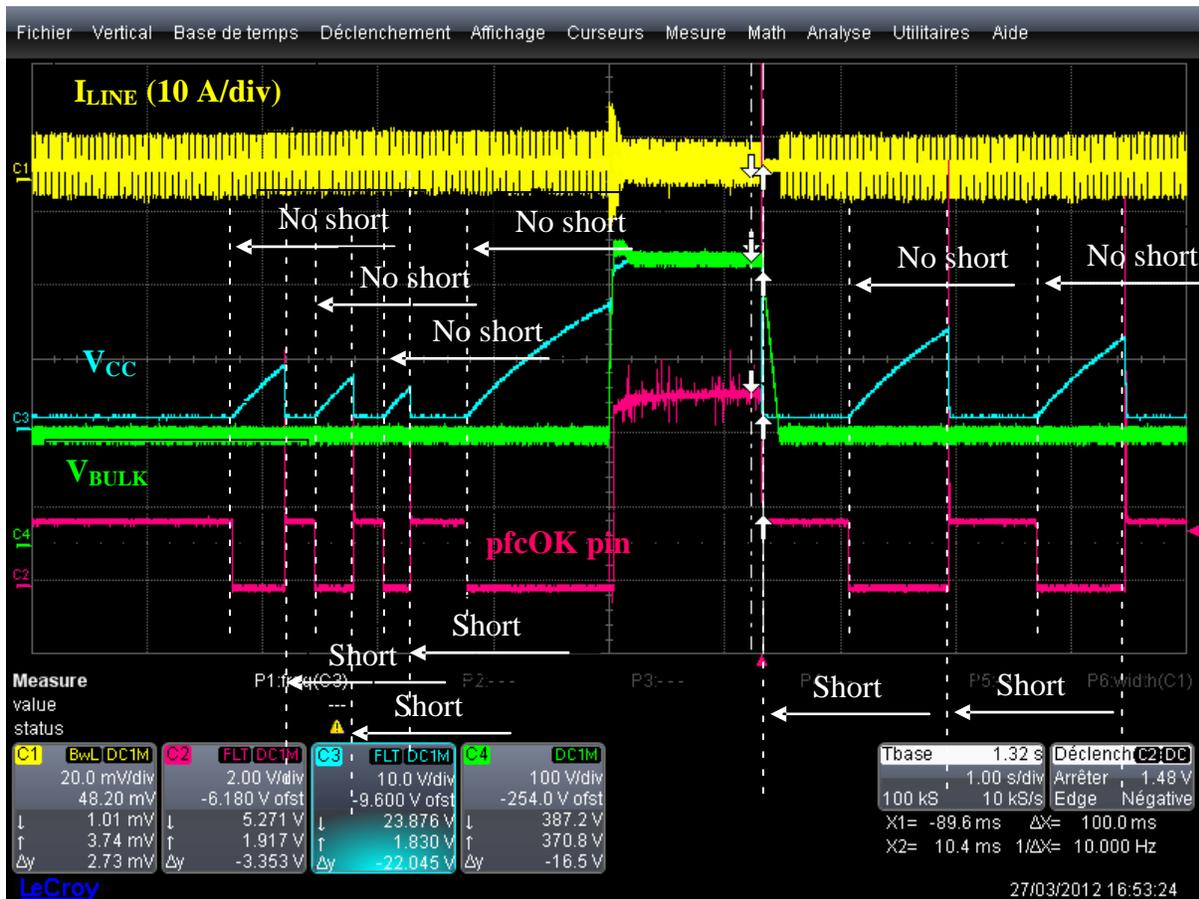
Figure 9. Short/No Short between the V<sub>CC</sub> and pfcOK Pins without a Power Source Applied to the V<sub>CC</sub> Socket @ 115 V, 60 Hz, 0.2 A Load
