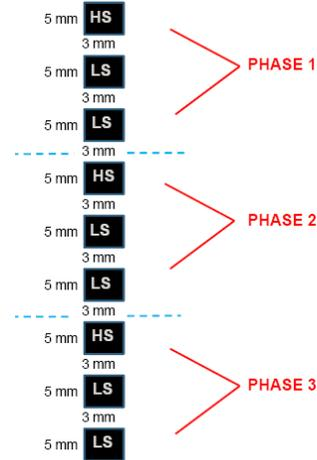
Figure 7. Example Layout for a 1 × 2 MOSFET Combination with a 3 mm Spacing
