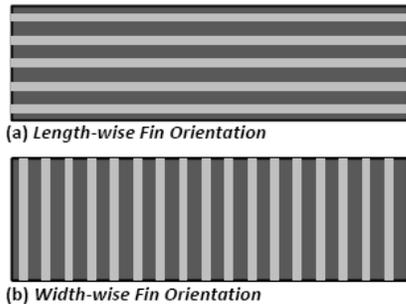
**Figure 2. Heat Sink Fin Orientation**
