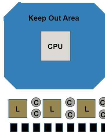
**Figure 5. Example Power Circuit Layout**
