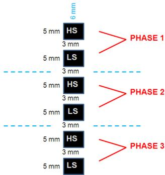
Figure 6. (a) Example Layout for 1 × 1 MOSFET Combination
