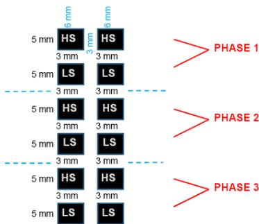
Figure 6. (b) Example Layout for a 2 × 2 MOSFET Combination
