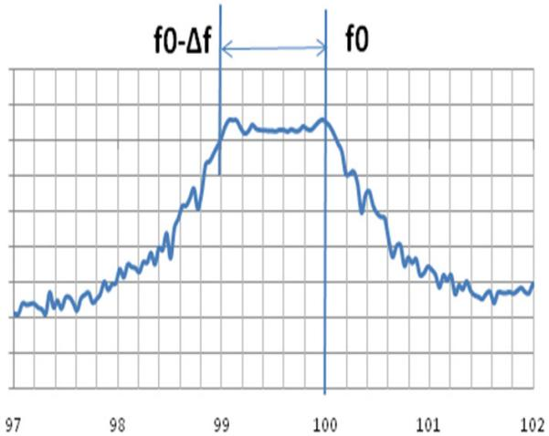
Figure 8. Down Spread (Spectrum Analyzer Plot)
