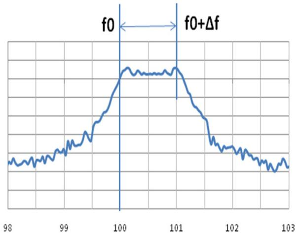
Figure 10. Up Spread (Spectrum Analyzer Plot)
