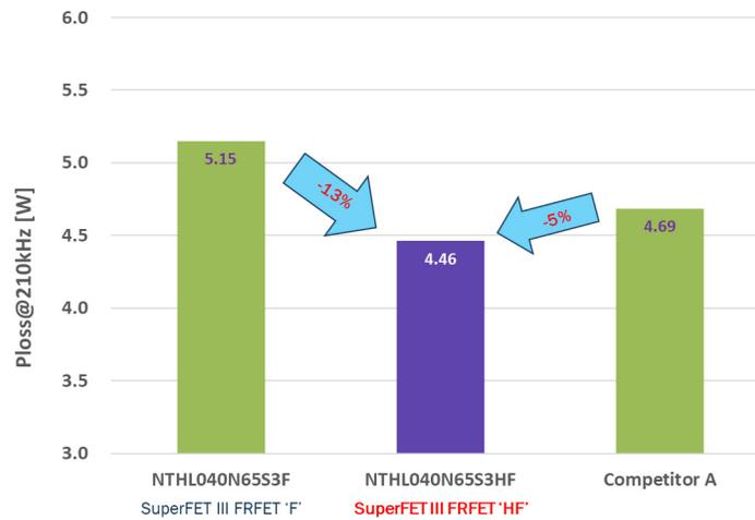
Figure 16. Power Loss Comparison: SUPERFET III FRFET F vs HF vs Competitor under in Two-level FB LLC of EV Charging Module
