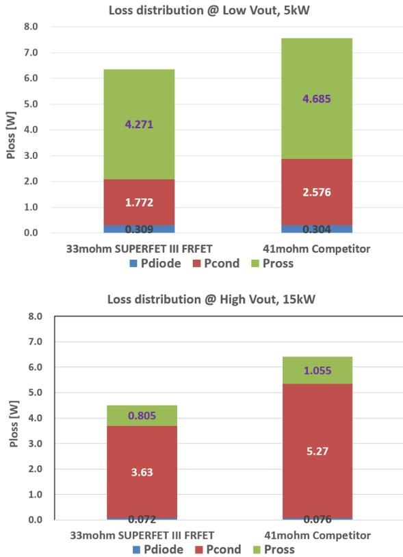
**Figure 13. Power Loss Distribution under Light Load and Full Load in Two-level FB LLC of EV Charging Module**
