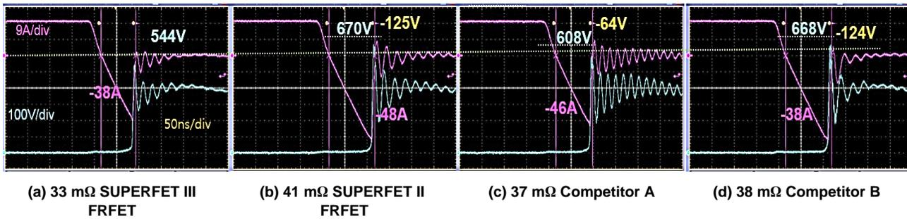
Figure 6. Comparisons of Reverse Recovery Behavior of Fast Recovery SJ MOSFETs under  $I_{SD} = 20 \text{ A}$ ,  $di/dt = 800 \text{ A}/\mu\text{s}$ ,  $V_{DS} = 400 \text{ V}$
