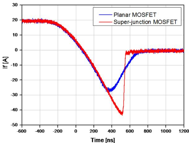
Figure 1. Reverse Recovery Behavior Comparison between Planar MOSFET and Super-junction MOSFET under  $V_{DD} = 400$  V,  $di/dt = 100$  A/ $\mu$ s,  $I_{SD} = 20$  A
