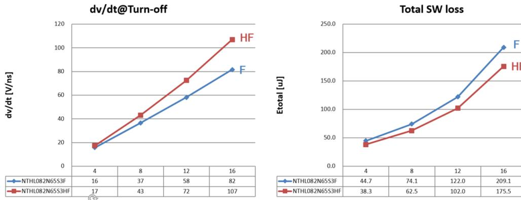
Figure 15. Comparisons of Turn-off Switching Characteristics: 82 mW SUPERFET III FRFET F and HF version under  $V_{DD} = 380\text{ V}$ ,  $V_{GS} = 10\text{ V}$ ,  $R_G = 4.7\ \Omega$
