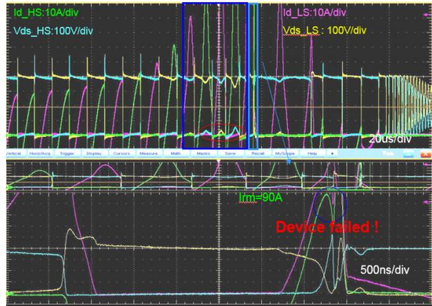
Figure 5. Waveforms of Power MOSFETs in LLC Resonant Converter at Short-Circuit Condition
