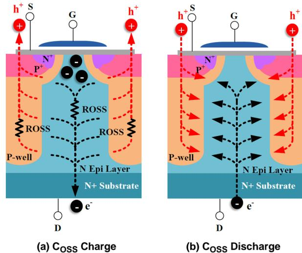
Figure 7.  $C_{OSS}$  Charge and Discharge of SJ MOSFET, Electron ( $e^-$ ) and hole ( $h^+$ ) Currents and Charge Pockets (Black and Red)
