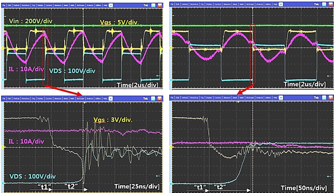
(a)  $P_{OUT} = 5 \text{ kW}$ : 200 V / 25 A / 207 kHz, above resonant frequency ( $f_s > f_r$ )
