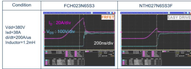
**Figure 3. Body Diode Reverse Recovery Comparison between 650 V SUPERFET III FRFET vs EASY Drive under  $V_{DD} = 380$  V,  $I_{SD} = 38$  A,  $di/dt = 200$  A/ $\mu$ s,  $T_j = 25^\circ$ C**
