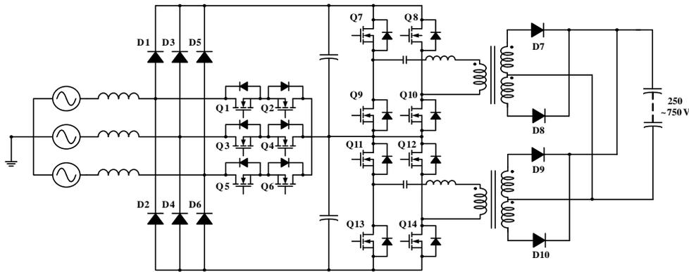
Figure 11. Power Stage of EV Charging Module : 3 phase Vienna PFC and Two Level Full-bridge LLC Resonant Converter
