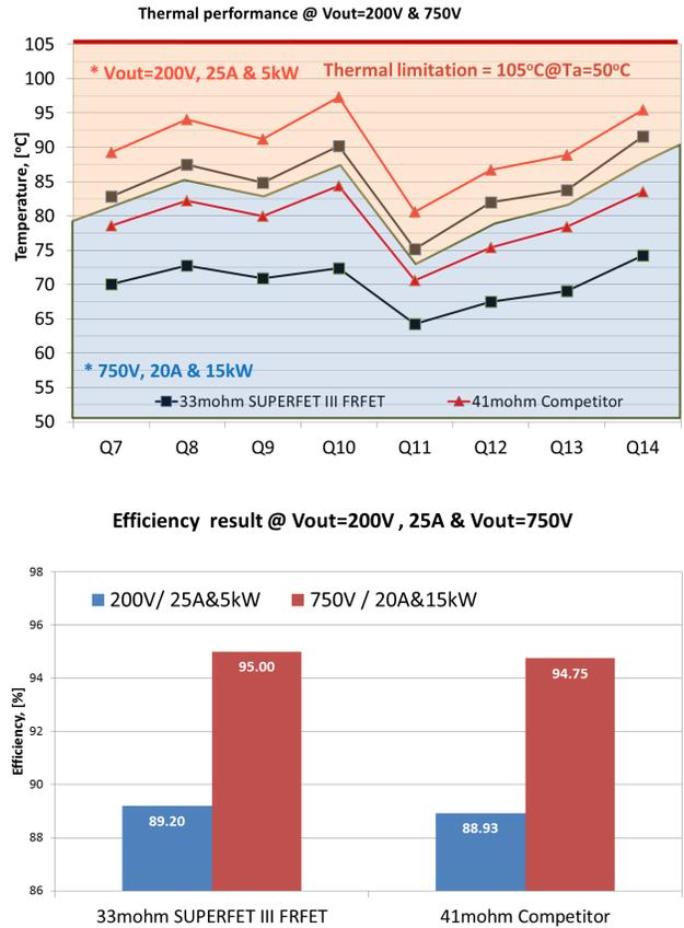
**Figure 14. Thermal and Efficiency Comparison in Two-level FB LLC of 15 kW EV Charging Module**
