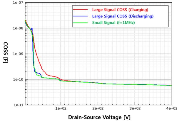
Figure 8. Comparison between Small Signal  $C_{OSS}$  (green line) and Large Signal  $C_{OSS}$ (red and blue lines)
