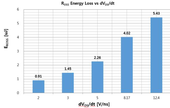
Figure 10. Energy Losses of SJ MOSFET during  $R_{OSS}$  Energy Loss vs Switching  $dV_{DS}/dt$  during Charging and Discharging [0~400 V $_DS$ ]
