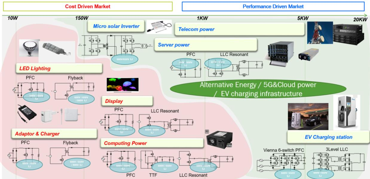
Figure 2. Target Application for 600 V ~ 800 V Super-Junction MOSFETs
