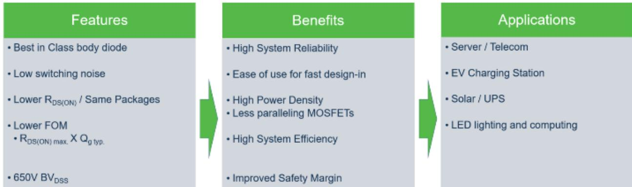
The SUPERFET III FRFET technology can provide low  $R_{DS(ON)}$  and the best-in-class body diode for lower conduction loss, and increased reliability in many AC-DC SMPS applications, which often require high power density, high system efficiency and high reliability.
