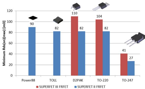
**Figure 4. Minimum  $R_{DS(ON)}$  (Max.) in different Packages of Power MOSFETS**
