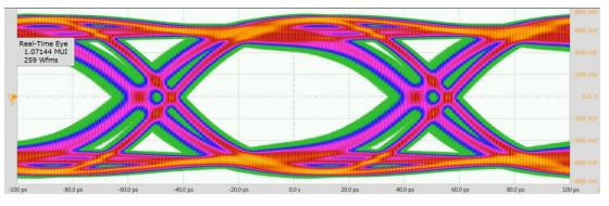
Figure 10. Eye Diagram Using Too Much Equalization
