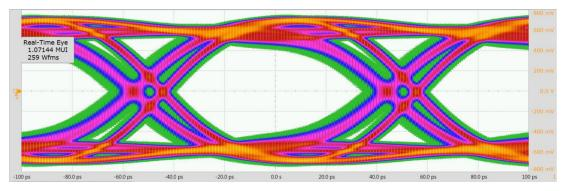
Figure 14. Eye Diagram with Distortion from Driving Signal Past Compression Point
