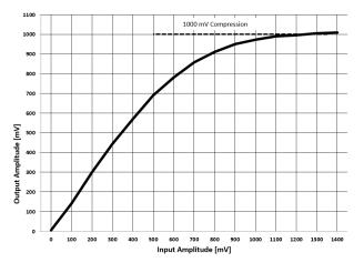
Figure 3. Output Compression – Input vs. Output Voltage
