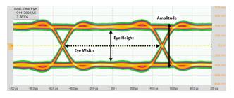
Figure 4. Eye Diagram Key Measurements
