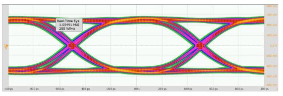
Figure 12. Eye Diagram Using No Flat Gain
