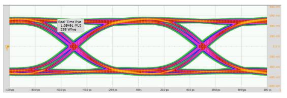
Figure 9. Eye Diagram Using Correct Equalization
