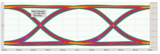
Figure 13. Eye Diagram Using Positive Flat Gain
