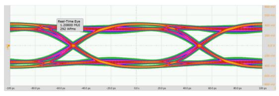
Figure 11. Eye Diagram Using Negative Flat Gain
