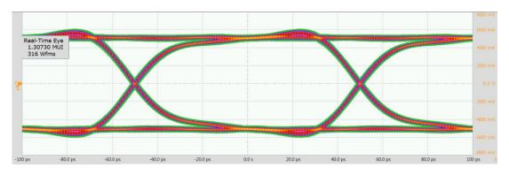
Figure 6. Eye Diagram of Signal before Loss
