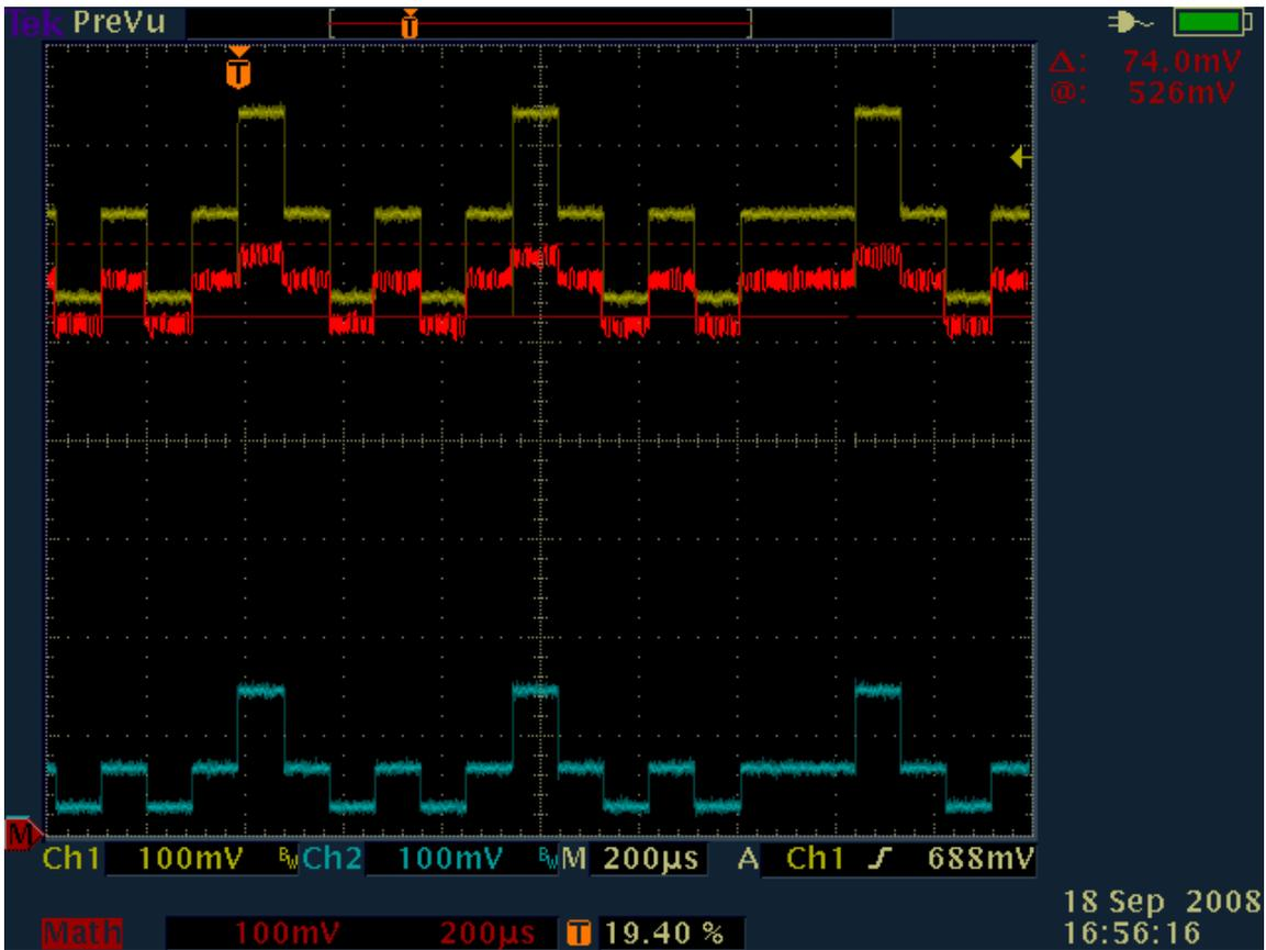
Figure 8. Typical D+/D- Waveforms for 3-current Device
