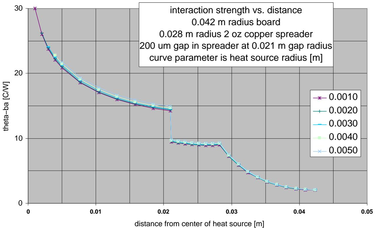
**Figure 17. Temperature Profile ( $^{\circ}\text{C}/\text{W}$ ) of 50x50 mm, 70 um Thick Copper Spreader on a 76x76 mm FR4 Board; Spreader has 200 um Discontinuity at a 21 mm Radius from the Heat Source**
