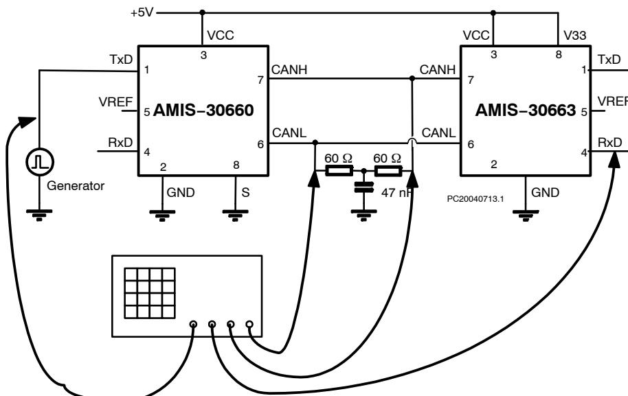
Figure 1. Measurement Setup
