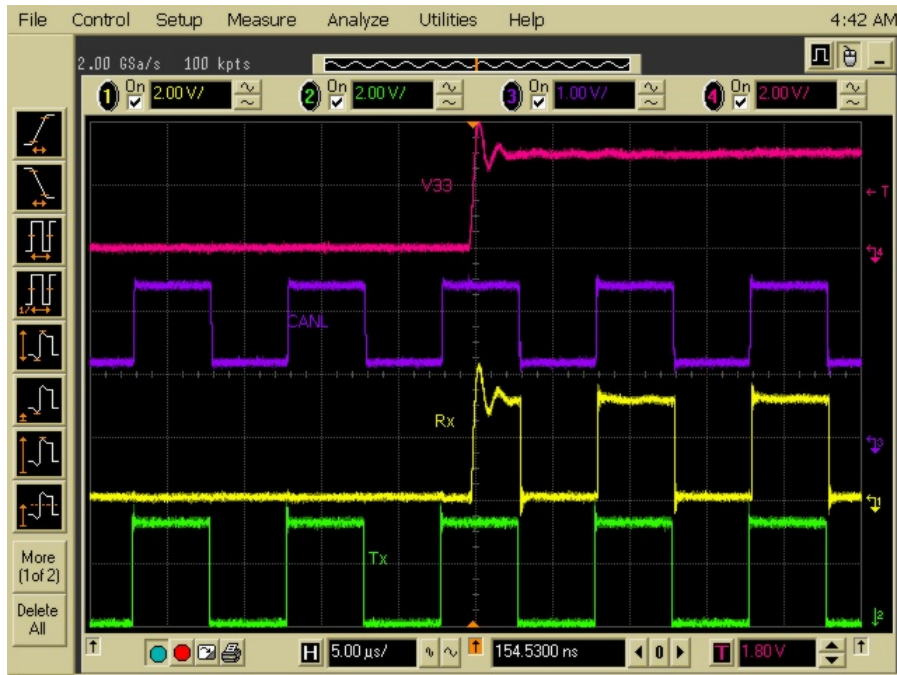
Figure 5. S is Close → V33 Transient at Recessive State (Tx = 1)
