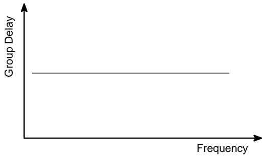
Figure 13. An idealized flat group delay across frequency. This is a result of a constant rate change of the system's phase angle across frequency.
