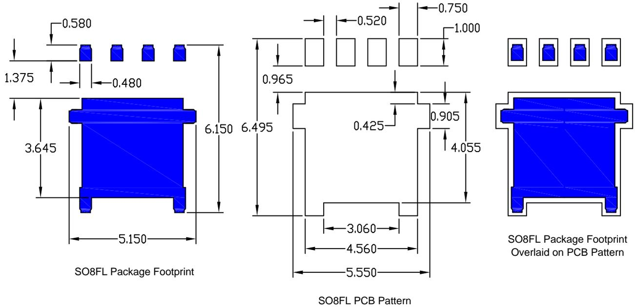
**Figure 4. Printed Circuit Board Layout Using Non-solder Masked Defined I/O Pads**
