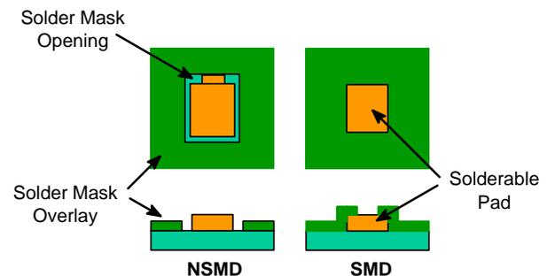
Figure 3. Comparison of NSMD vs. SMD Pads
