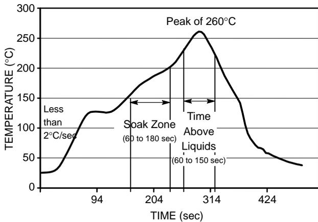
**Figure 7. Typical Reflow Profile for Standard Pb-free Solder**
