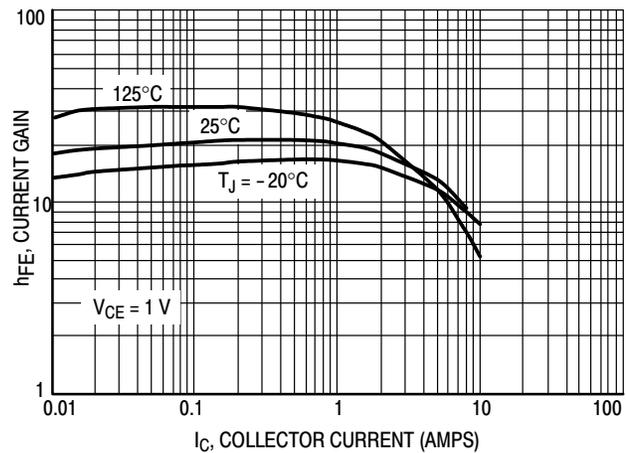
Figure 2. Typical Gain Curves for the Planar MJW18010
