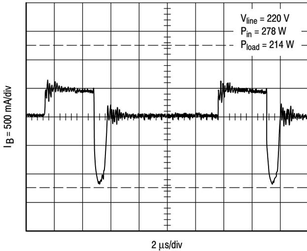
Figure 5. Base-Drive Waveforms of the MJW18010 in a 300-W Power Supply
