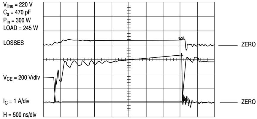
Figure 12. Losses in the Power MOSFET
