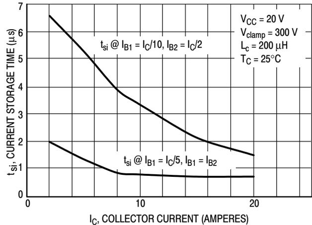
**Figure 3. Collector Current Storage Time as a Function of  $I_C$  and Base Bias (MJW18010)**
