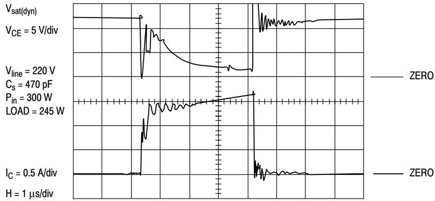
Figure 13. Dynamic  $V_{CE(sat)}$  of the Bipolar Transistor
