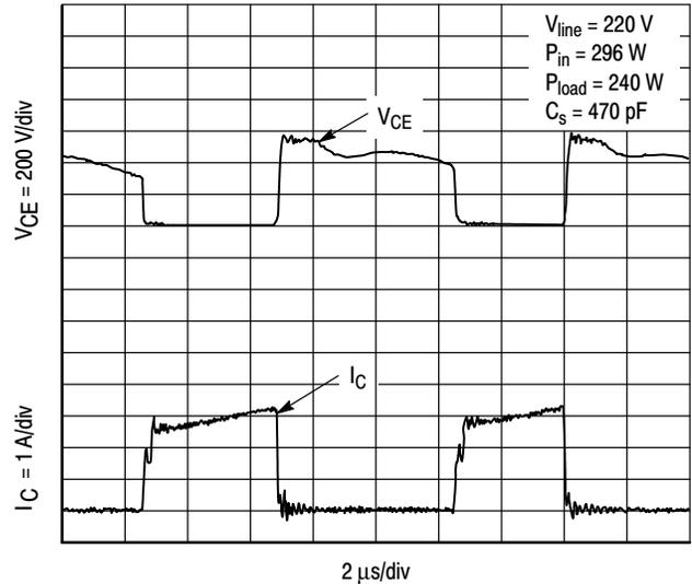
Figure 6. Collector Current and Collector-to-Emitter Voltage Waveforms of the MJW18010 in a 300-W Power Supply
