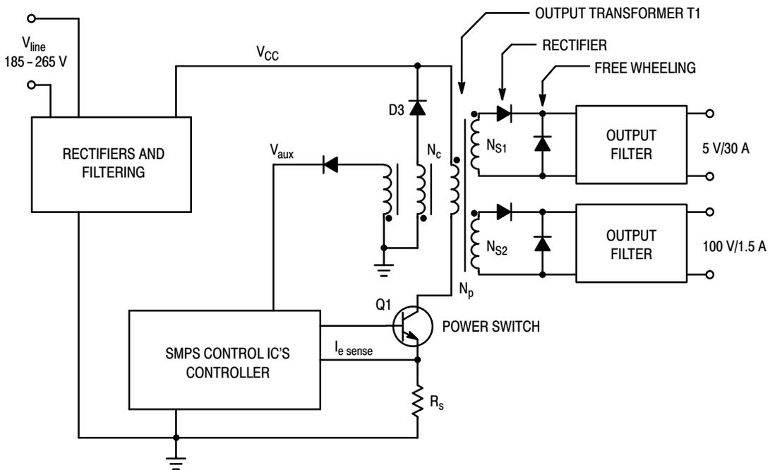
**Figure 8. SWITCHMODE Power Supply Block Diagram**
