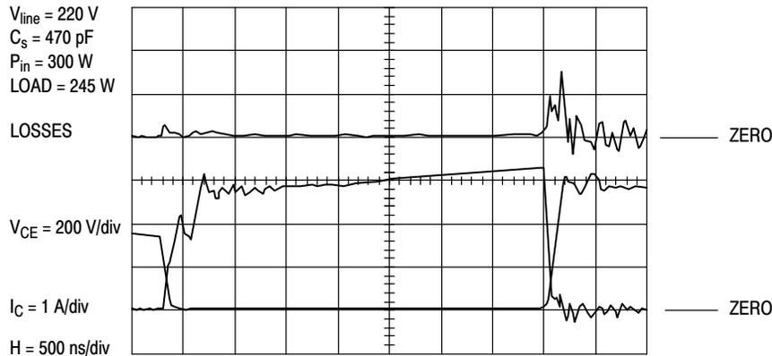
**Figure 11. Losses in the Bipolar Transistor**
