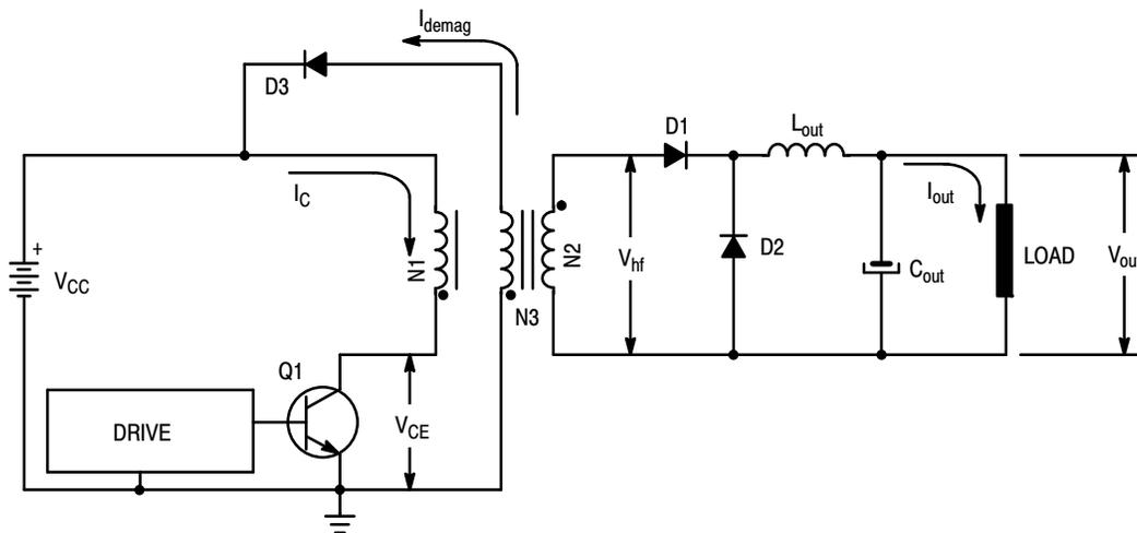
Figure 7. Basic Forward Converter Topology
