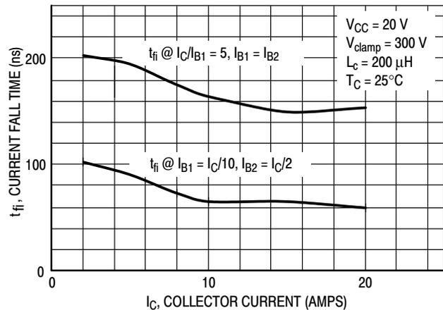
**Figure 4. Collector Current Fall Time as a Function of  $I_C$  and Base Bias (MJW18010)**
