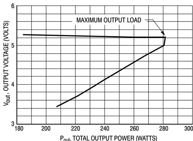
**Figure 10. Foldback Characteristic of the 300-W, 100-kHz Converter**
