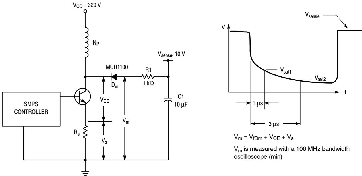
Figure 14. Dynamic On-voltage Test Circuit
